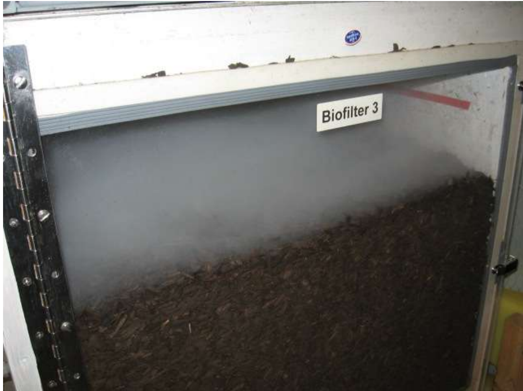
Figure 3.6. Smoke passing through the compost.
