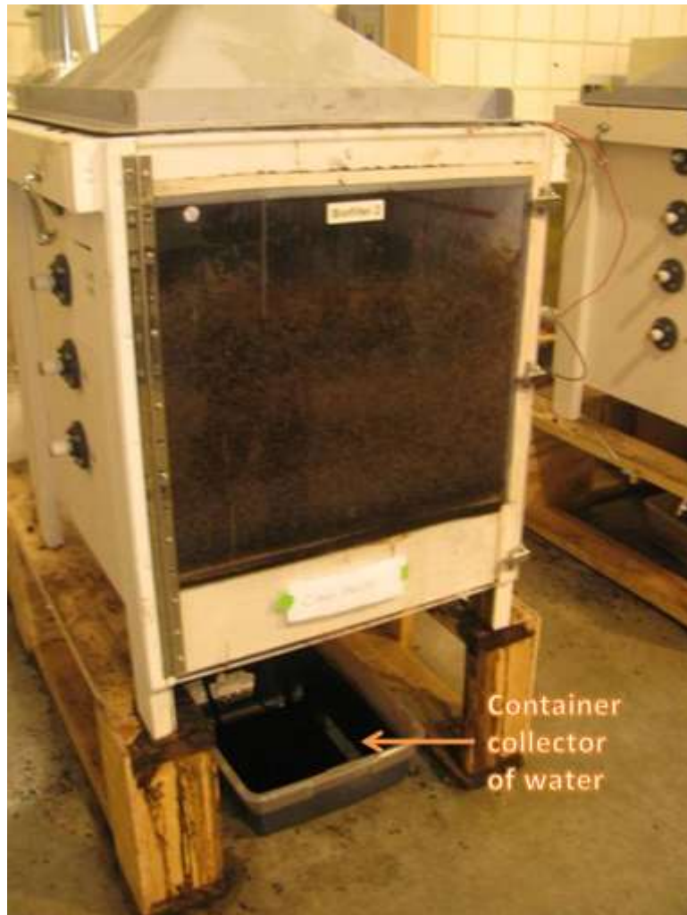
Figure 3.32. Container collecting water from the biofilter.
