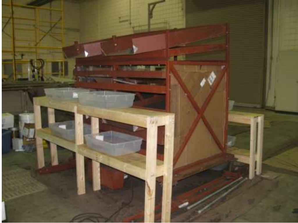
Figure 3.14. Sieve shaker machine with the add-on component.
