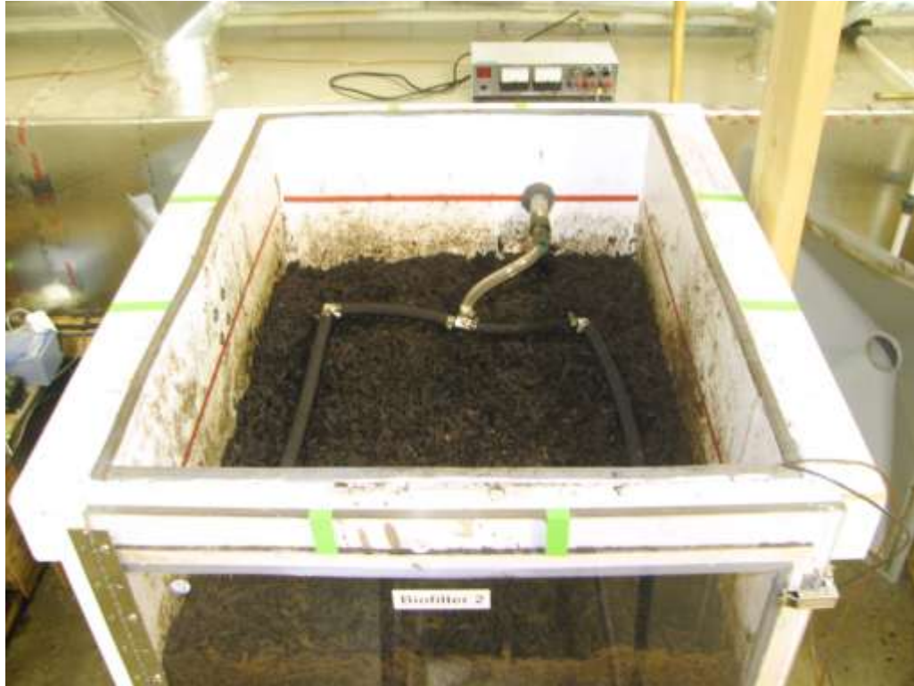
Figure 3.31. Hose located at the upper position in the biofilter.
