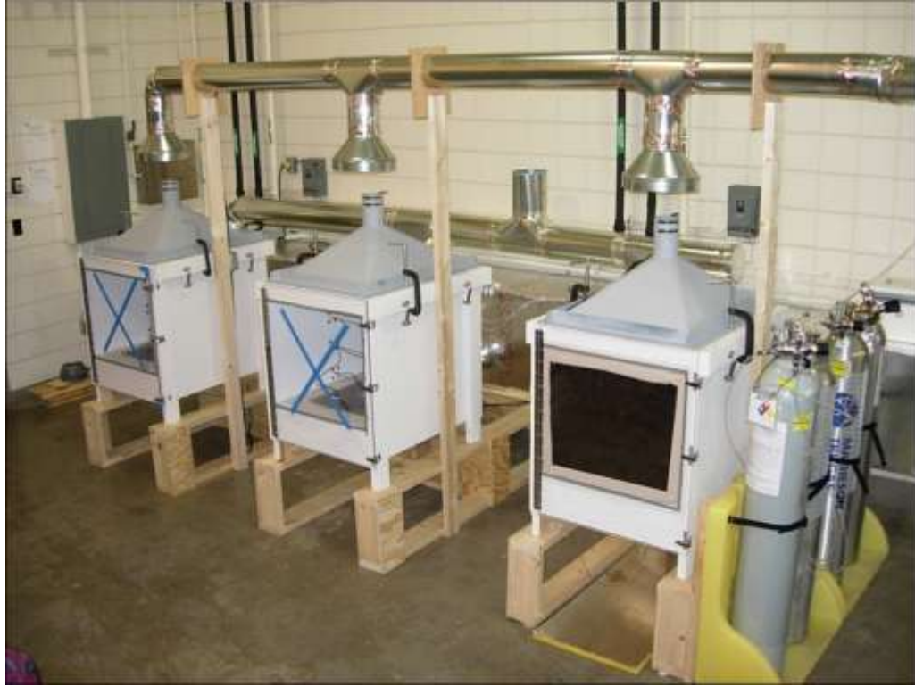
Figure 3.1. Biofilter chambers in the Agriculture Air Quality Laboratory (Sales, 2008).
