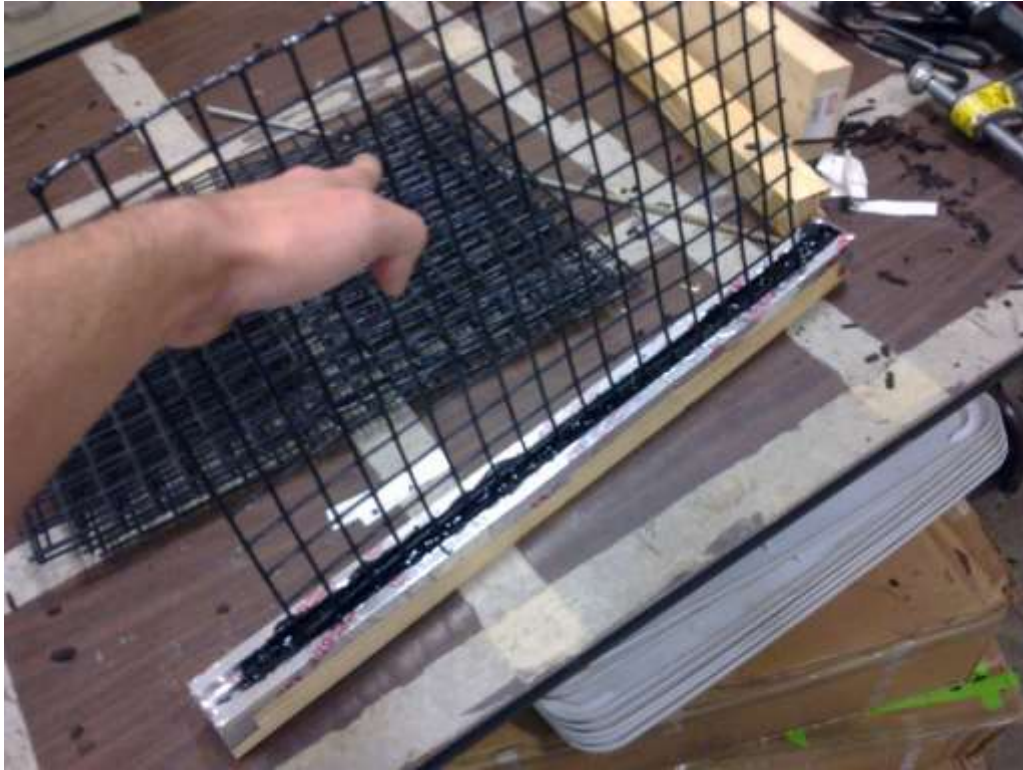
Figure A.3.2.1 Process of coating the tips of the grids for insulation with PlastDip®.
