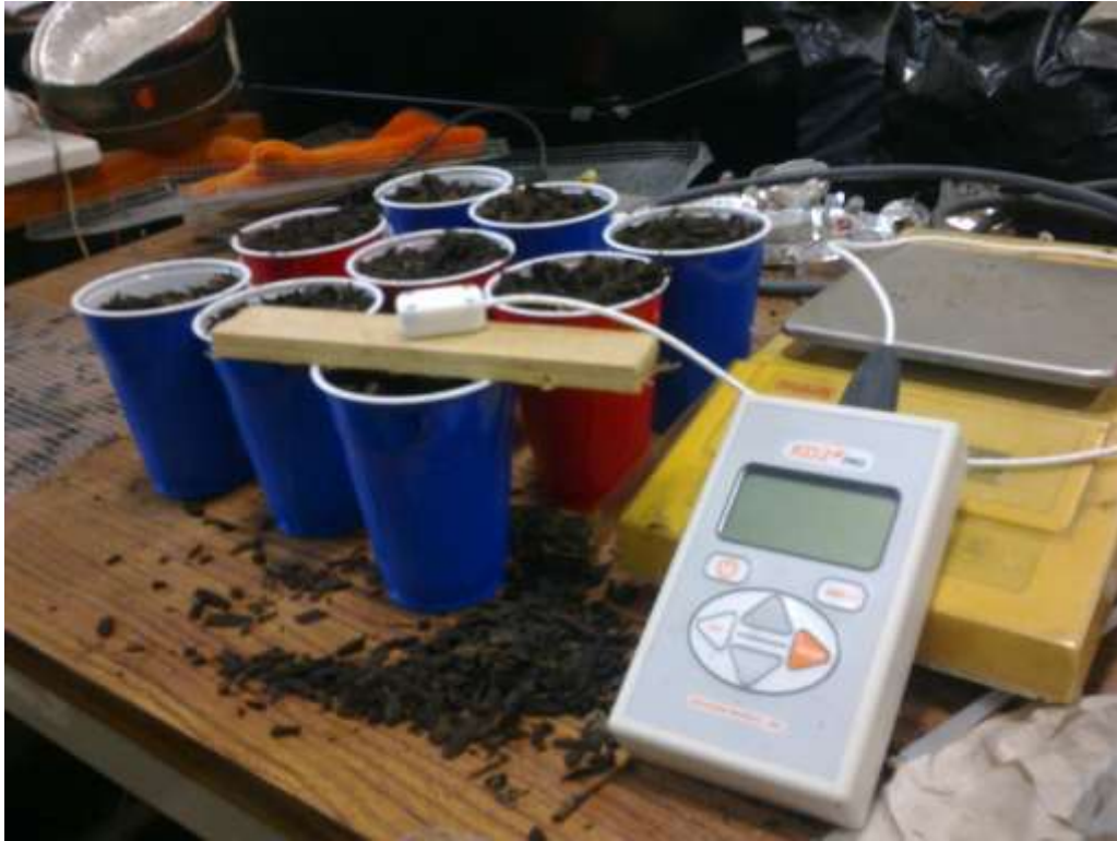
Figure 3.23. Thermal conductance probe tested for plywood wall effect.
