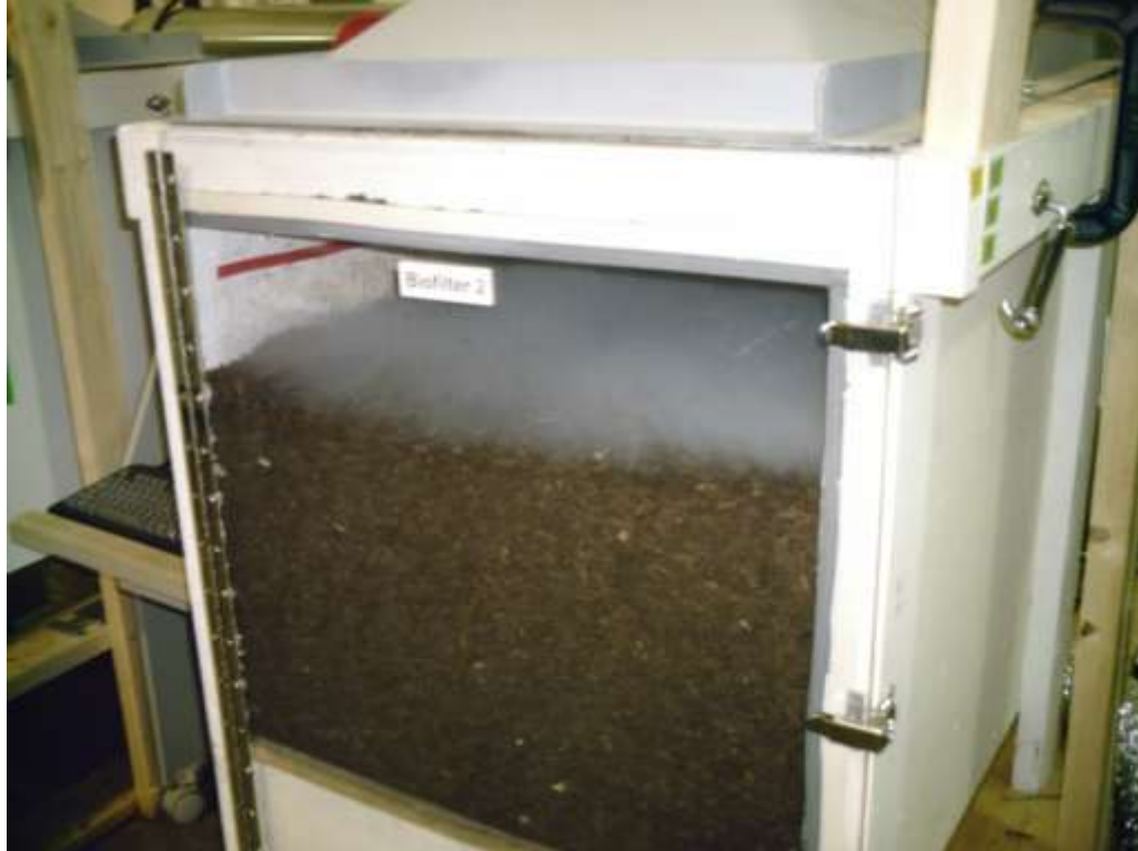
Figure 4.4. Smoke rising to the media surface.
