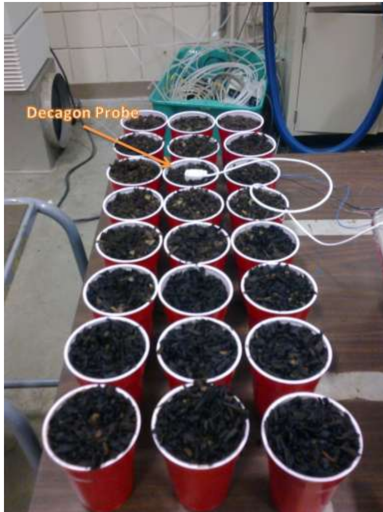
Figure 3.22. Decagon probe inserted into the compost.
