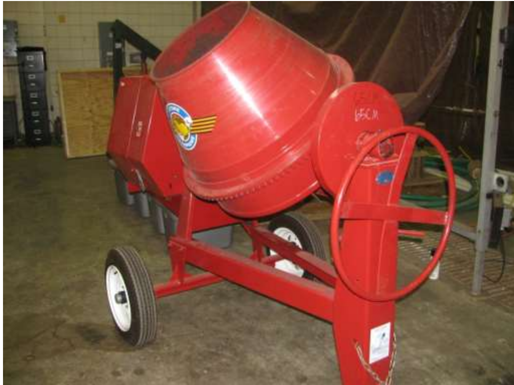
Figure 3.20. Concrete mixer used for mixing compost.
