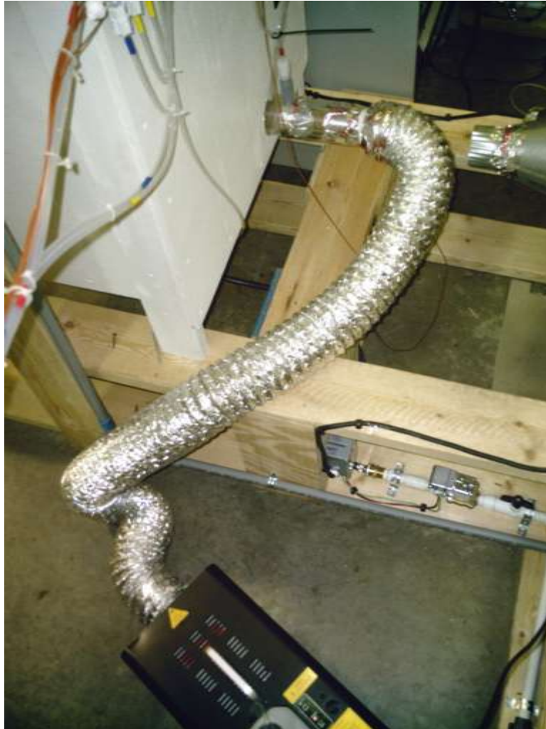
Figure 3.5. Smoke machine connected to the biofilter plenum
