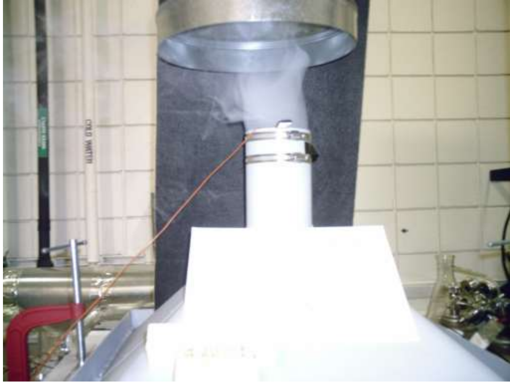
Figure 4.7. Showing back pressure over biofilter 3.
