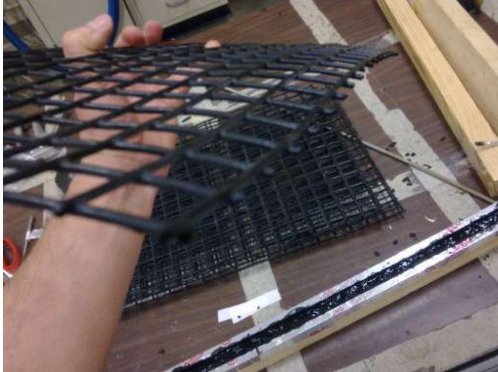
Figure A.3.2.2 Tips of the grids insulated with PlastDip®.
