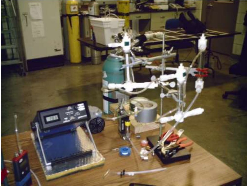
Figure 3.4. Setup of the flow meters connected in series with the pump (not shown) or the cylinder through the mass flow controller.
