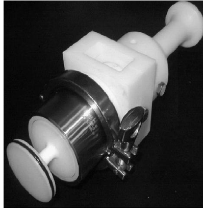
Figure 3.3 – The specially designed sampler for sampling curd and whey from the vat (Everard et al., 2008).
