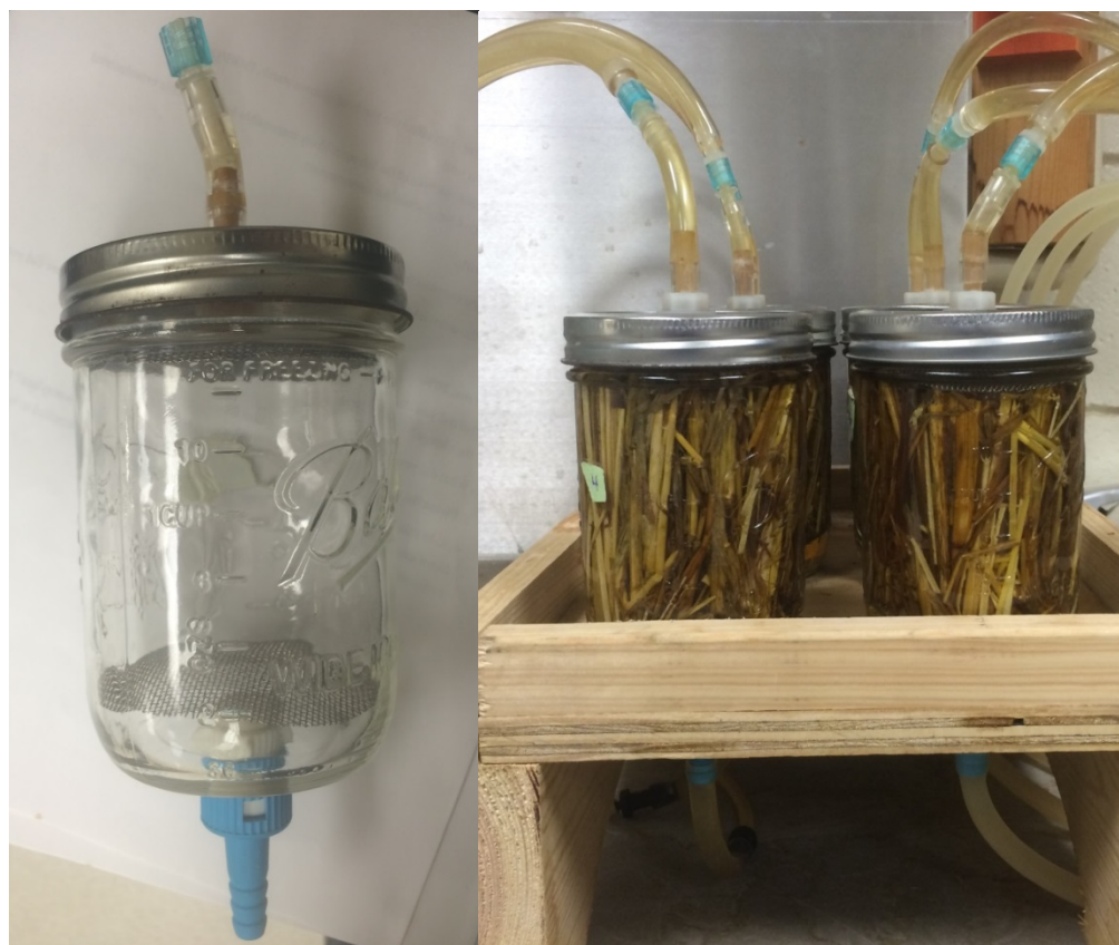
Figure 2: Up-flow Treatment Vessel left; Six Vessels in Use right
