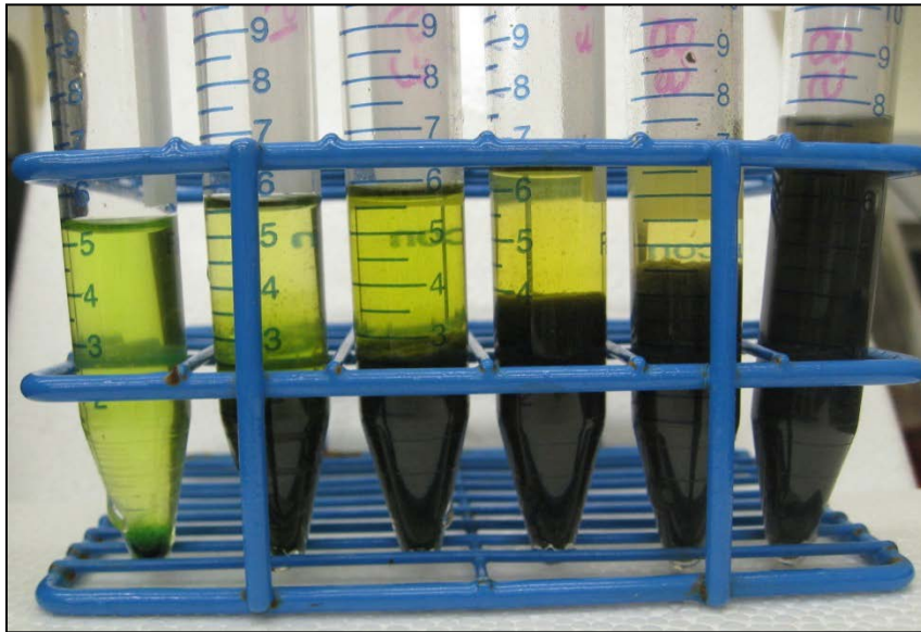
Figure 4-11 Sample tubes to perform chlorophyll extraction with varying manure volumes. From left to right the samples were no manure and 10 ml algae, 2 ml manure and 8 ml algae, 4 ml manure and 6 ml algae, 6 ml manure and 4 ml algae, 8 ml of manure and 2 ml algae, 10 ml manure.
