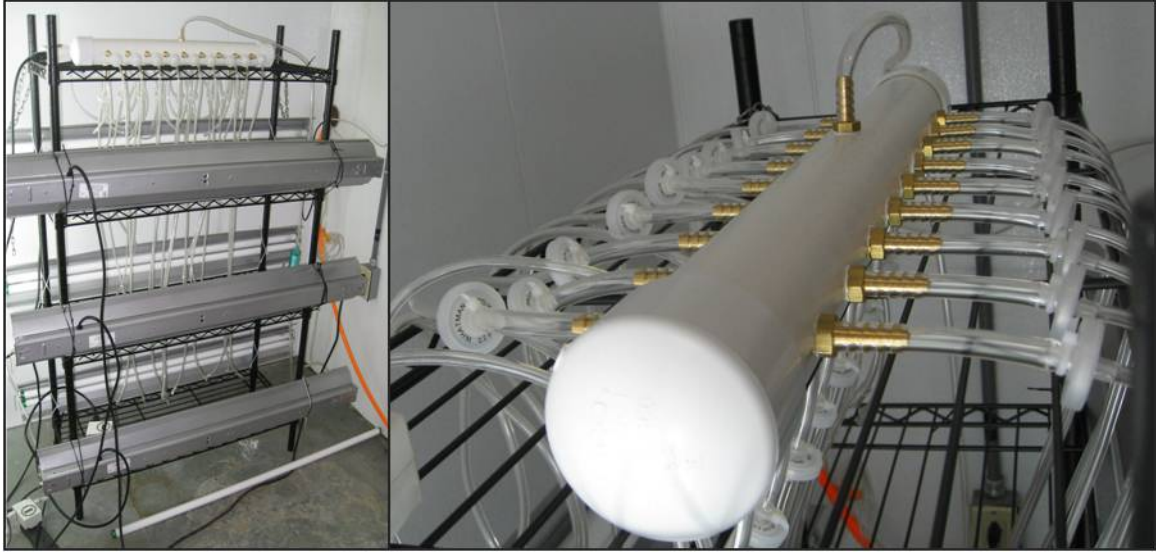
Figure 4-1 Shelving unit with lights and manifold.
