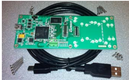
Figure 3.6 ADIS 16228 SPI to USB communication kit
