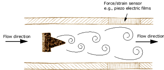
Figure 1.6 Karman effect and the principle of vortex flow meter (Yoder, 2010).
