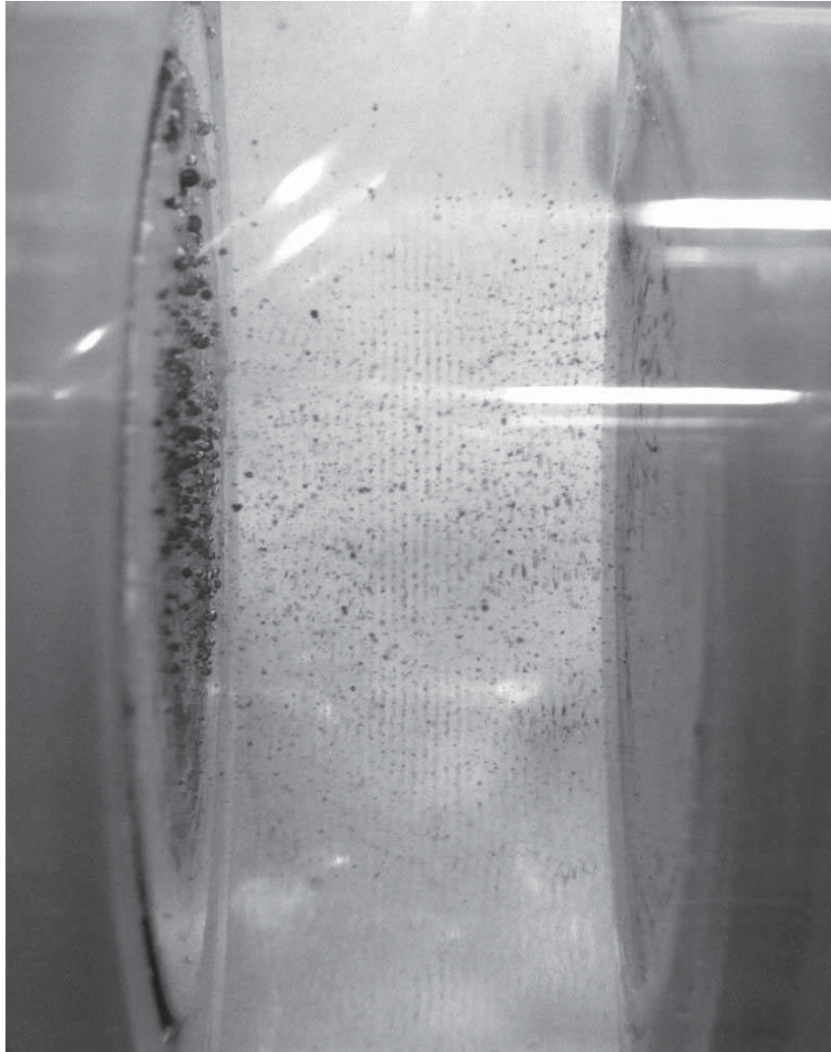
Figure 4.1 Close-up view of concentrated red 10 \mu m polystyrene particles (shown without reticulated mesh)
