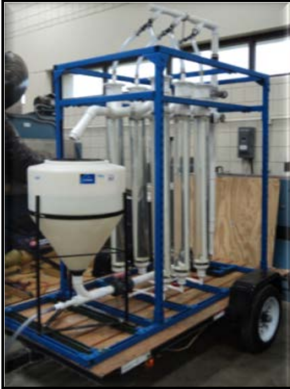
Figure 3.5: Picture of the trailer scale reactor, 188 L total volume.
