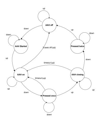
Figure 5: Automatic Attitude Hold State Diagram [2], [22]
