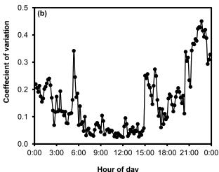
Figure 2. 24-h patterns for (a) total water usage of the plant and (b) coefficient of variation of total water usage based on data collected in (a). The flow rates in (a) were normalized by dividing the water flow readings by the maximum flowrate observed at 2 P.M. on Friday.
