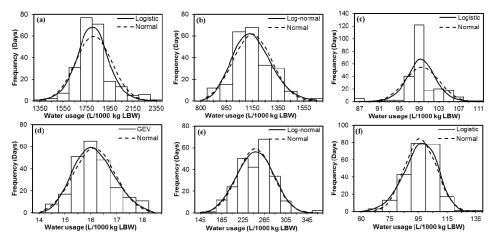
Figure 4. Water use variability for (a) processing water, (b) overnight use, (c) pre-evisceration wash, (d) organic acid spraying, (e) carcass wash, and (f) thermal pasteurization.
