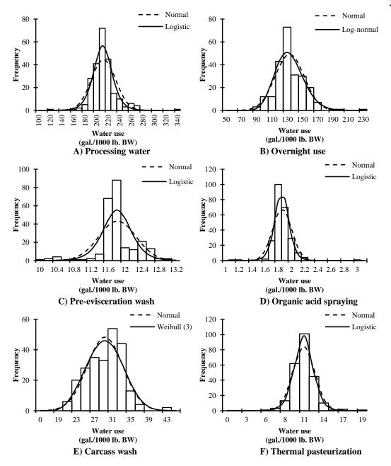
Figure 4.3: Water use distributions for processing water, overnight use and antimicrobial interventions. (Frequency is the day count for each water use)
