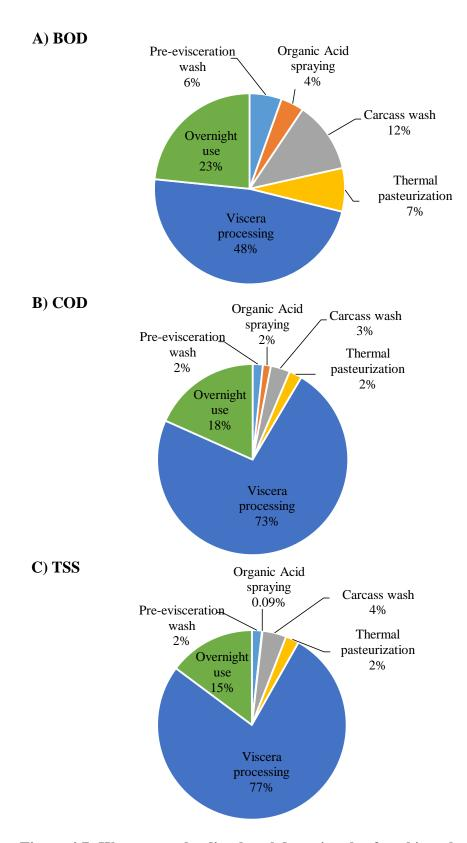
Figure 4.7: Wastewater loading breakdown in a beef packing plant
