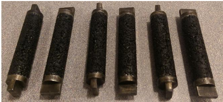
Figure 3.3. Fine aggregate matrix specimens with holders.
