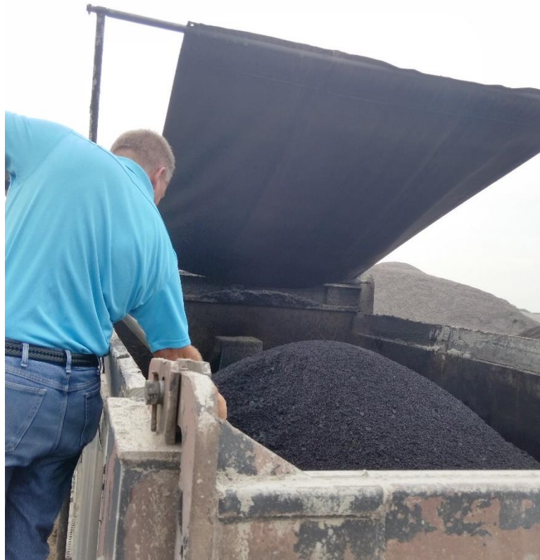
Figure 3-1 Mixture collection from a dump truck at asphalt concrete plant
