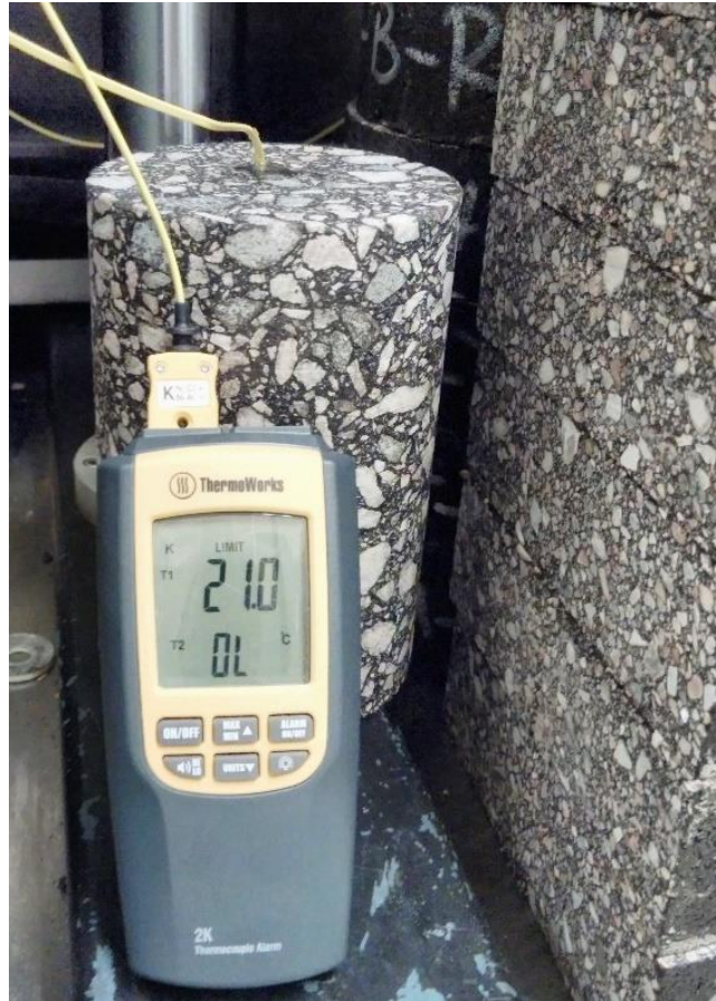
Figure 3-3 Reading temperature of specimens
