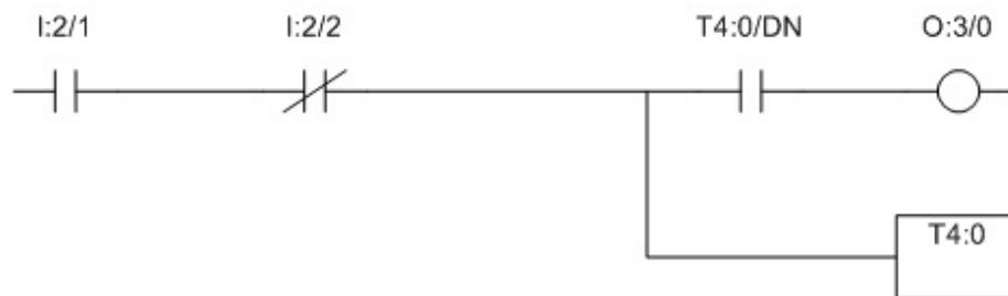
Figure 4.14: Ladder Logic: Elimination of Race Condition
