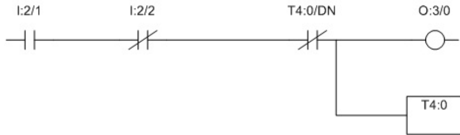
Figure 4.11: Race Condition: Ladder Logic Incorrect
