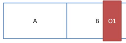
Figure 32: Polygon A and Polygon B are partially visible to each other under Type A partial visibility
