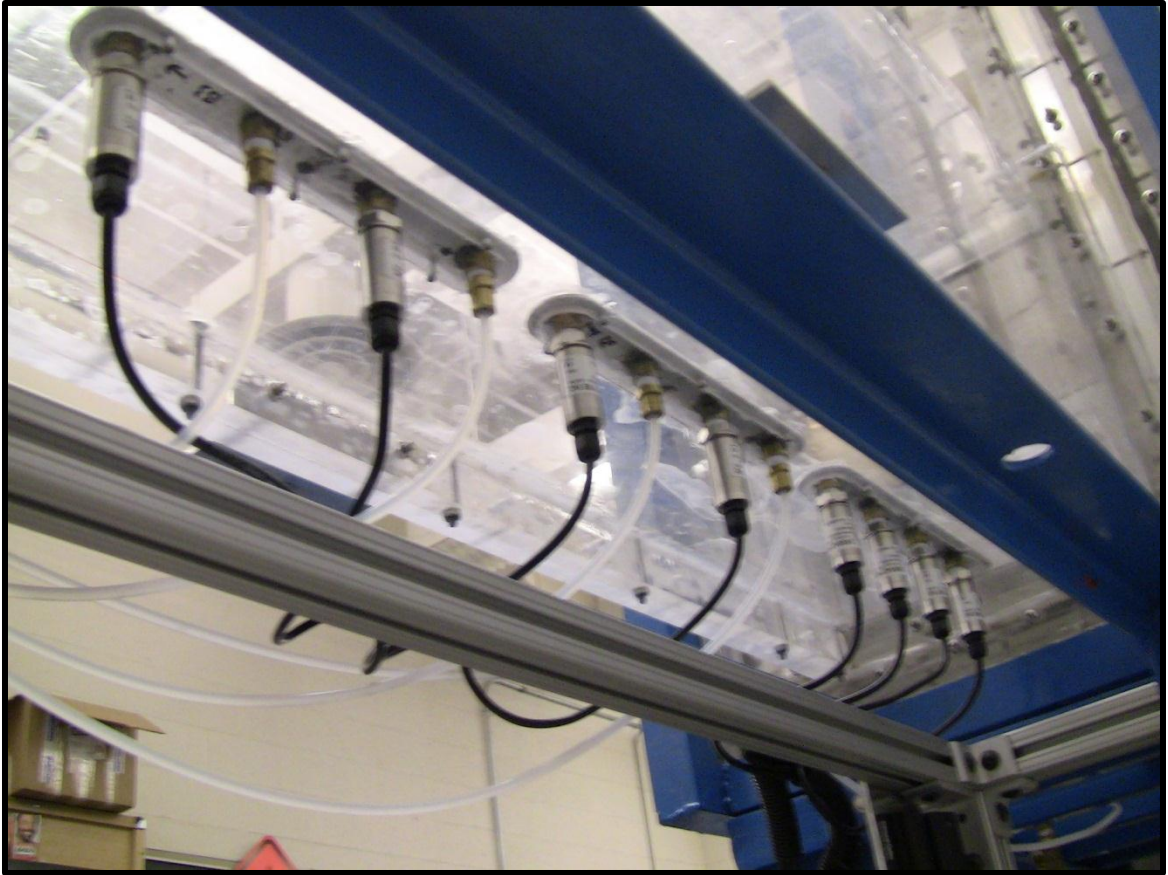
Figure 4-2 Pressure transducers and manometers installed in the slot inserts along the flume bed
