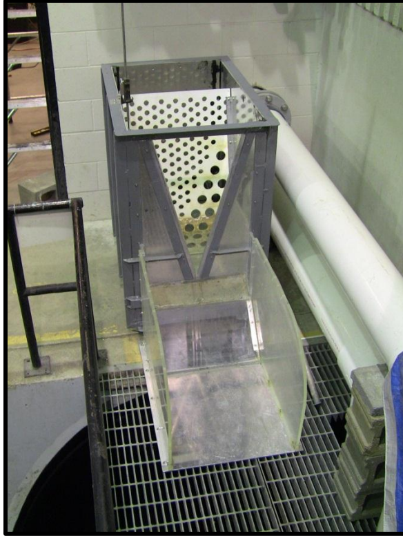
Figure 3-8 V-Notch weir tank
