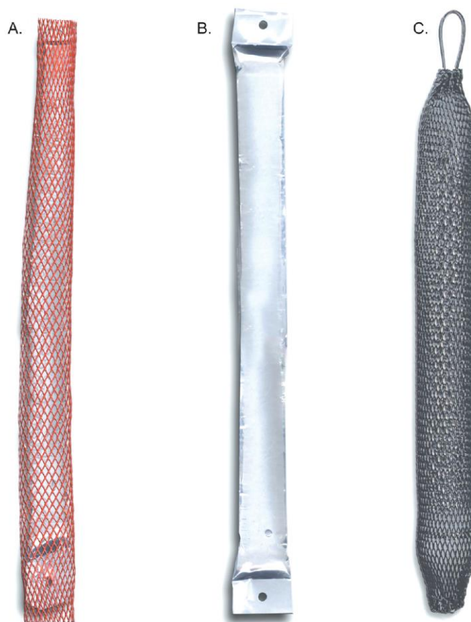
Figure 2-8 Passive Diffusion Bag Sampler (b) with protective mesh (a) & (c) (Vroblesky 2001a)
