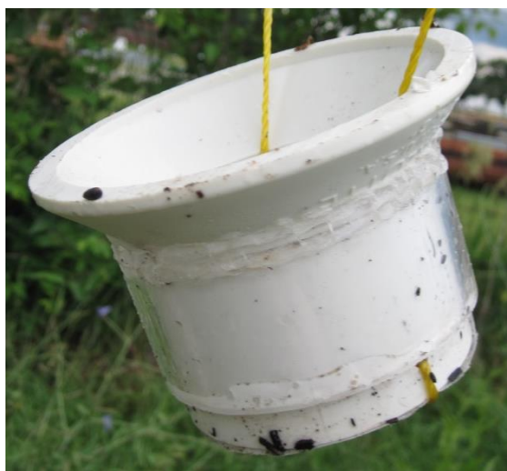
Figure 4-13 Bioretention Deployment Unit Influent Sampler Housing
