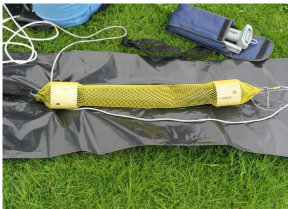
Figure 2-2 Regenerated Cellulose (Dialysis) Membrane Sampler (Imbrigiotta et al. 2007)
