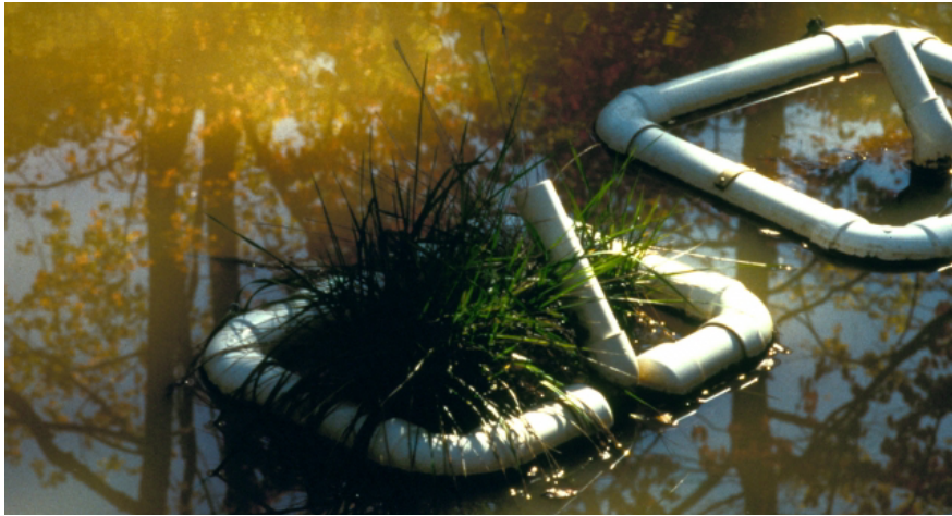
Figure 2-7 Overgrown Vegetation Restricting Movement of Skimmer (Faircloth 2010)
