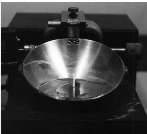
FIG. 7 Grooved Soil Pat in Liquid Limit Device
