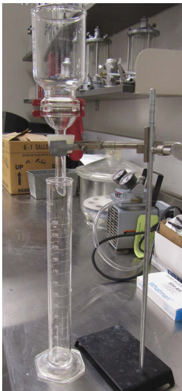
Figure 4.6: Filtration System with No Vacuum
