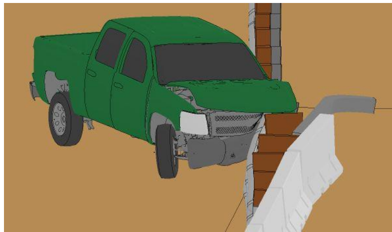
Figure 66. Vehicle Snag on Blockout for Impact Location No. 6 at 90 ms
