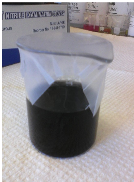
Figure 18: Stable GO suspension following Method 1
