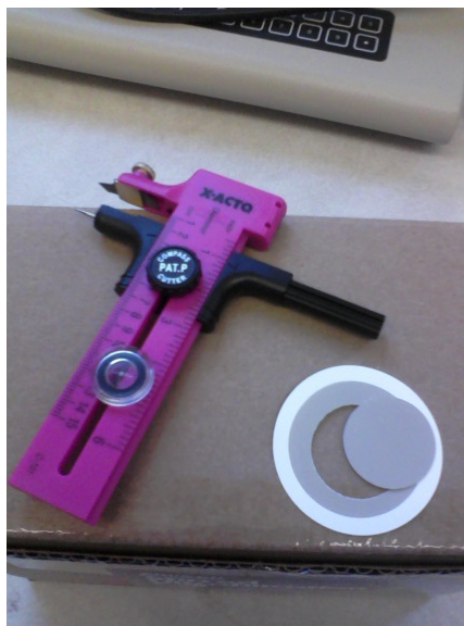
Figure 24: Membrane coated with GO cut to 25mm
