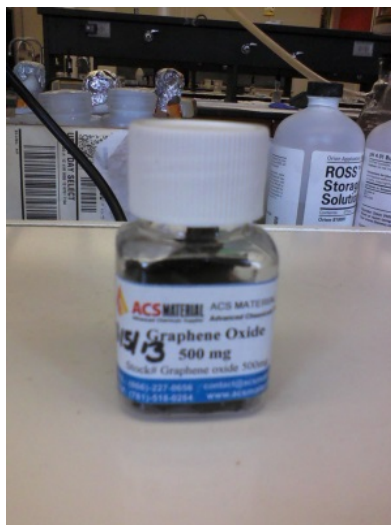
Figure 9: Purchased single layered graphene oxide
