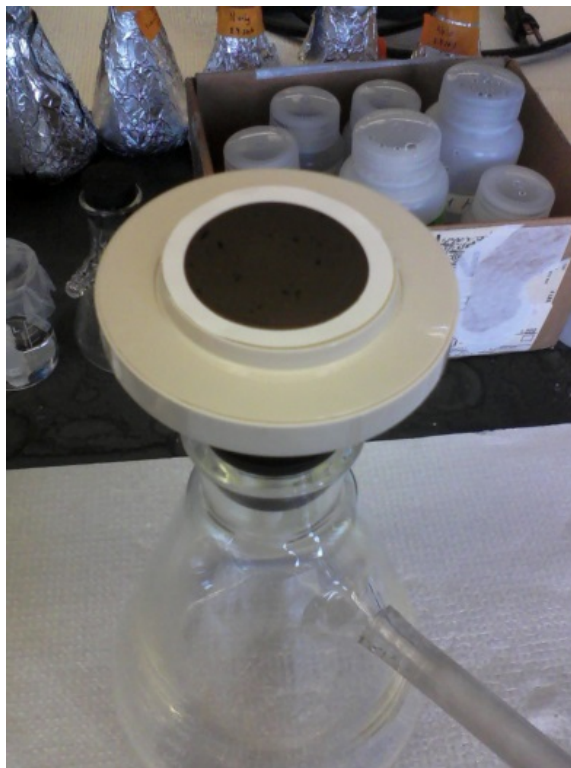
Figure 19: Membrane coated with GO following Method 1
