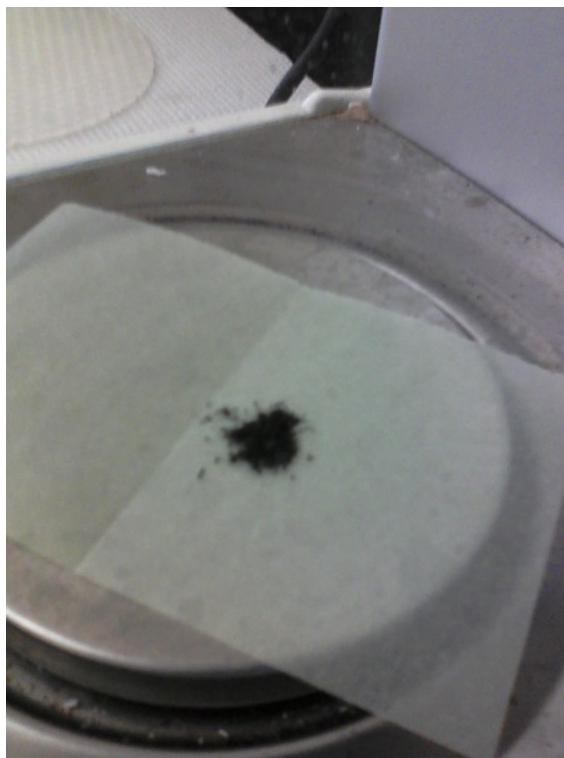
Figure 21: Crushed GO flakes
