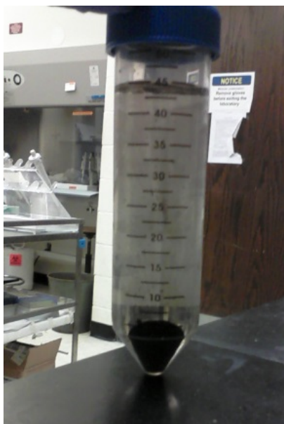
Figure 14: GO following centrifuge process
