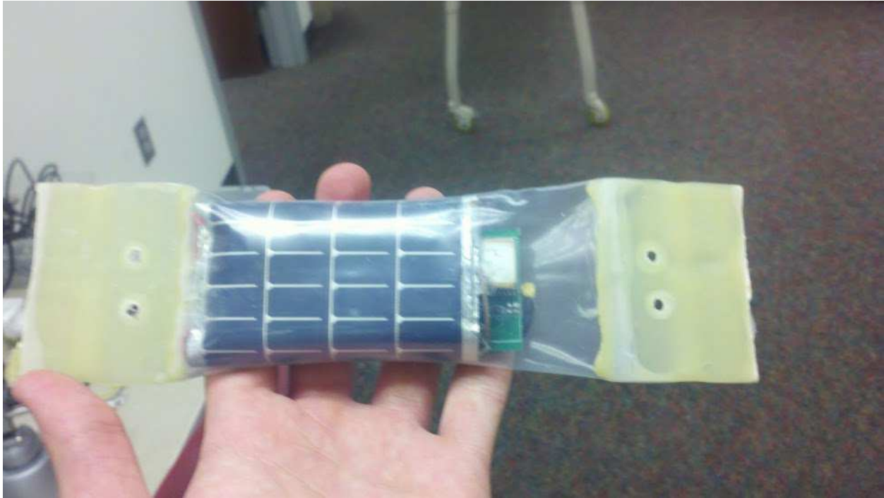
Figure 6.5: Flexible heat-shrink tubing being sealed with improved adhesive.
