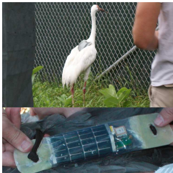
Figure 6.2: CraneTracker on captive Siberian Crane (top), close-up view (bottom).
