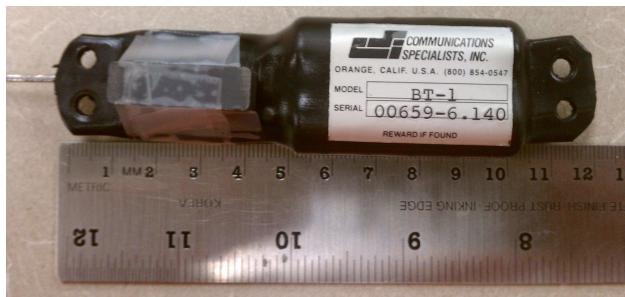
Figure 6.3: The VHF transmitter that inspired final enclosure design.
