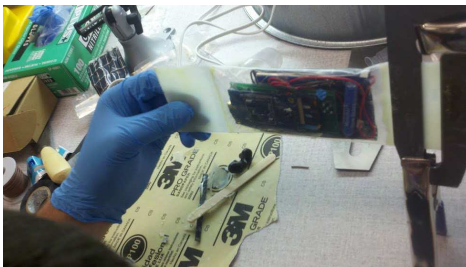
Figure 6.4: Flexible heat-shrink tubing being sealed with improved adhesive.
