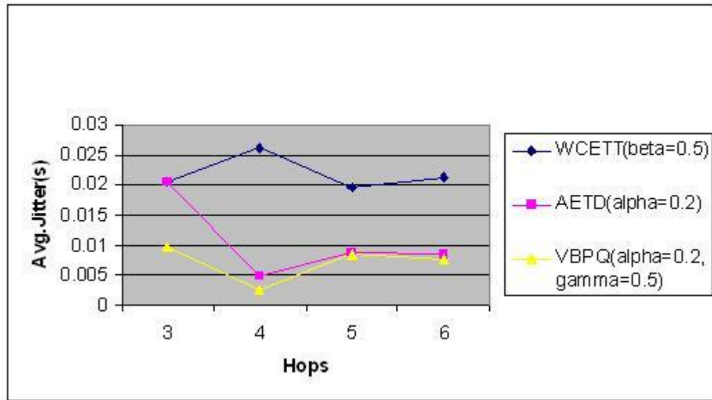
Figure 4.13 Multi Radio: Avg.Jitter Comparison of VBPQ, AETD and WCETT under delay-variation attack
