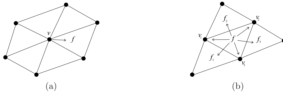
Figure 4.8 Connectivity of a triangular mesh: (a) each vertex has a pointer to one of its incident triangles; (b) each triangle has pointers to its three vertices and to the three adjacent triangles.
