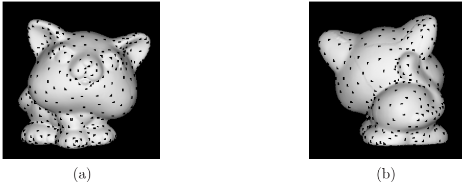
Figure 4.9 Sampling a cat model: front (a) and back (b) views of the model with a total of 550 sample vertices displayed as black dots on its surface.
