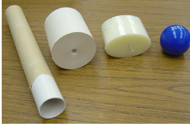
Figure 4.15 Algebraic objects used in experiments: two regular cylinders with diameters 50.4mm and 94mm, respectively, an elliptic cylinder with semimajor axis 50.8mm and semiminor axis 31.75mm, and a sphere with radius 33mm.
