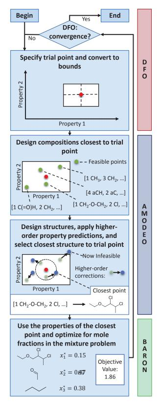
Figure 2.2: Mixture design algorithm
