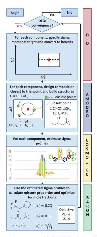
Figure 3.6: A pictorial representation of the COSMO-based mixture design algorithm
