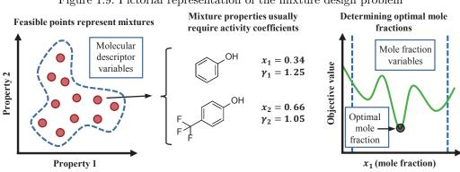
Figure 1.9: Pictorial representation of the mixture design problem
