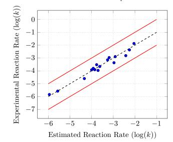
Figure 4.4: GC-estimated reaction rate vs. experimental reaction rate
