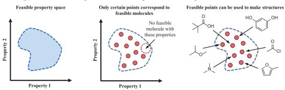
Figure 1.6: Pictorial representation of the problem of finding all feasible molecules
