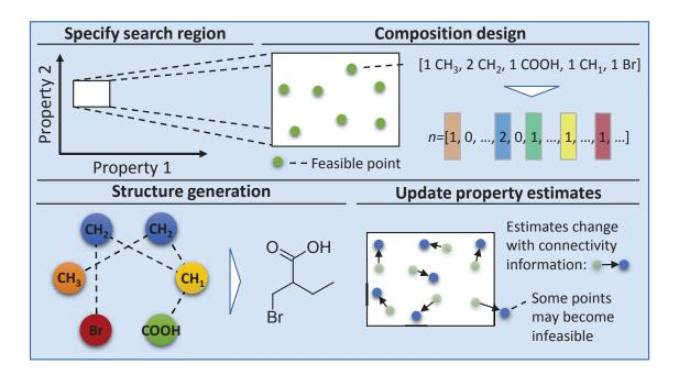
Figure 2.1: AMODEO framework for molecular design
