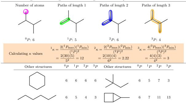
Figure 1.4: Getting  ${}^{i}P$  and calculating  ${}^{i}\kappa$  for an example molecule
