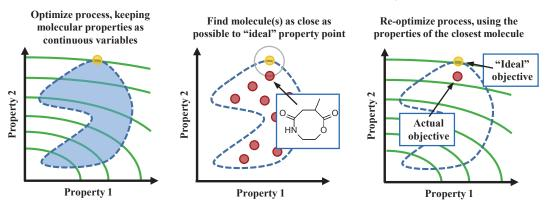
Figure 1.10: A decomposition approach to the integrated product/process design problem
