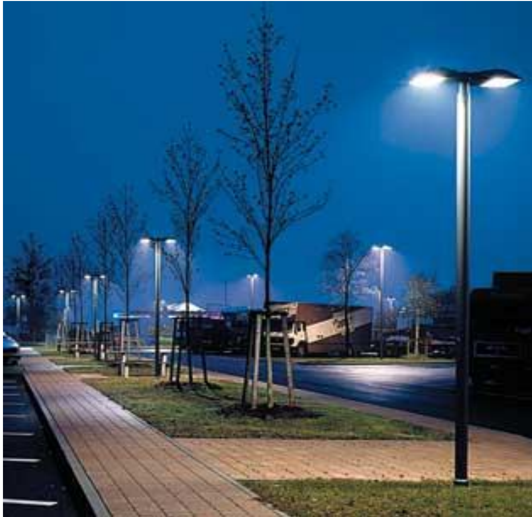
Figure 5-8. Example of CPTED-compliant lighting for pathways and parking areas
