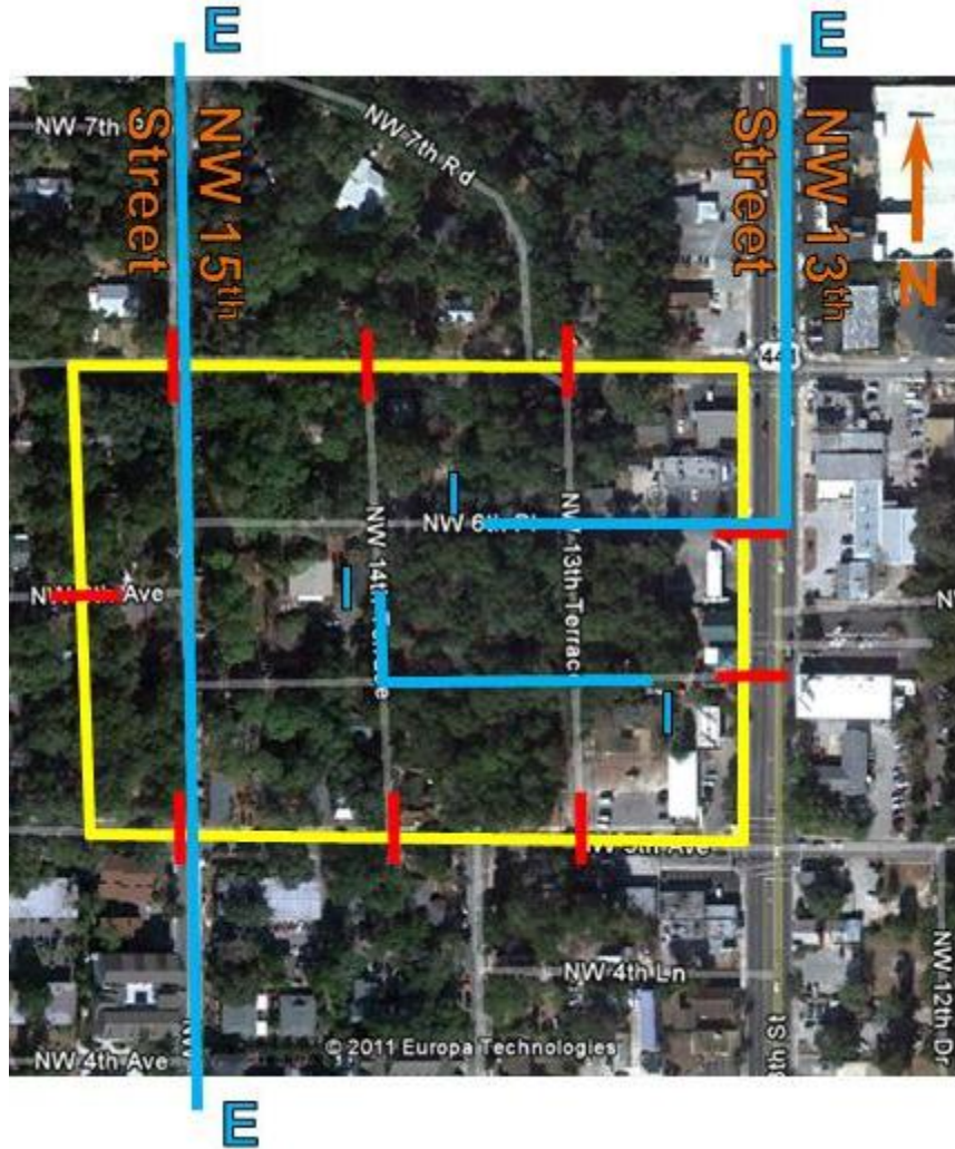
Figure 4-15. College Park Study Area travel patterns. The network cordon is seen in yellow. Cordon access points are marked in red. "I" denotes an internal origin or destination of a trip and "E" an external origin or destination.
