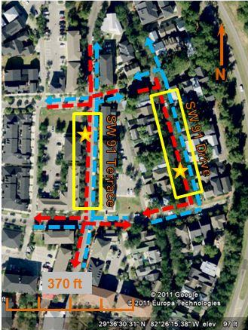
Figure 3-6. Haile Village Center speed study strategy. Selected study segments on SW 91 Terrace and SW 91 Drive are shown within the yellow boxes. The locations from which I recorded speeds are shown as gold stars. The blue dotted lines show the northbound movements of vehicles that were recorded, while the red dotted lines show the southbound movements of vehicles that were recorded.
