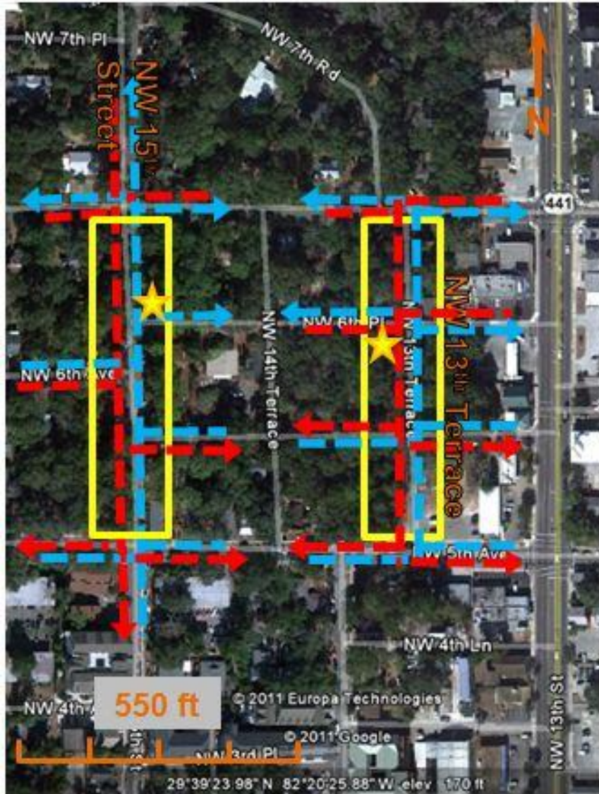
Figure 3-7. College Park speed study strategy. Selected study segments on NW 15 th Street and NW 13 th Terrace are shown within the yellow boxes. The locations from which I recorded speeds are shown as gold stars. The blue dotted lines show the northbound movements of vehicles that were recorded, while the red dotted lines show the southbound movements of vehicles that were recorded.
