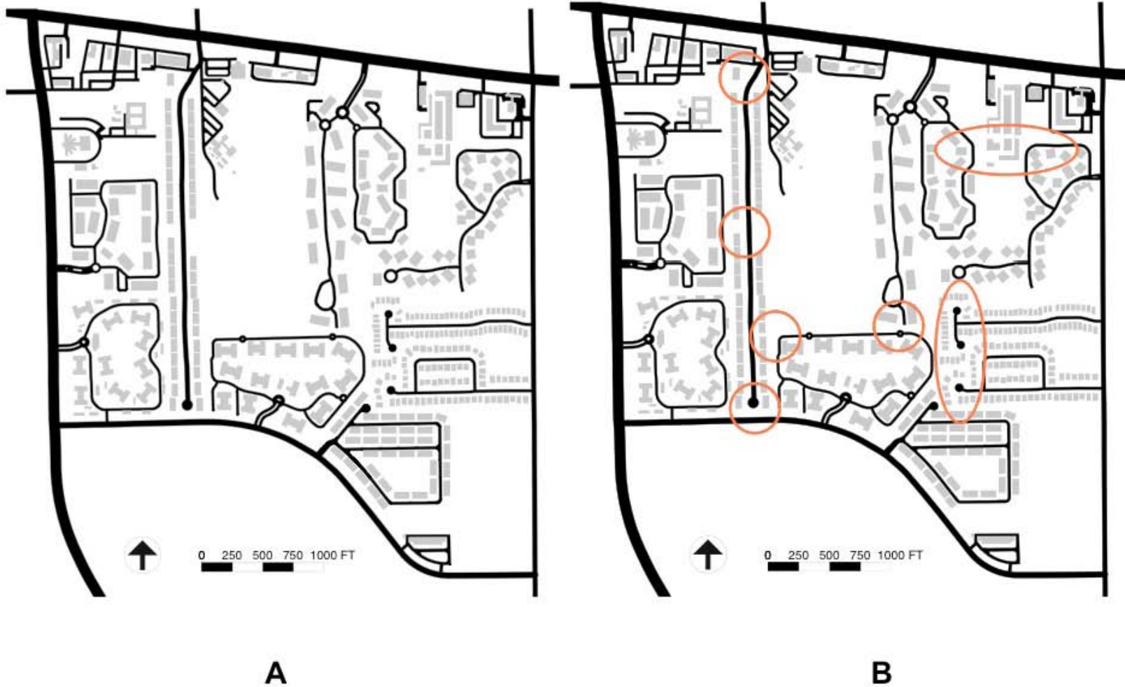
Figure 4-13. Deficiencies of a multifamily subdivision: Lack of walkable block structure. A) The contained pods of a sprawling multifamily development are evident in the existing figure ground. B) Missed opportunities for connectivity are indicated by orange circles.
