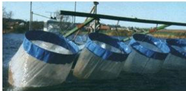
Figure 2-10. A set of bongo nets is hauled in and inspected by National Oceanic and Atmospheric Administration (NOAA) Ship McArthur crew members (NOAA, 2007).
