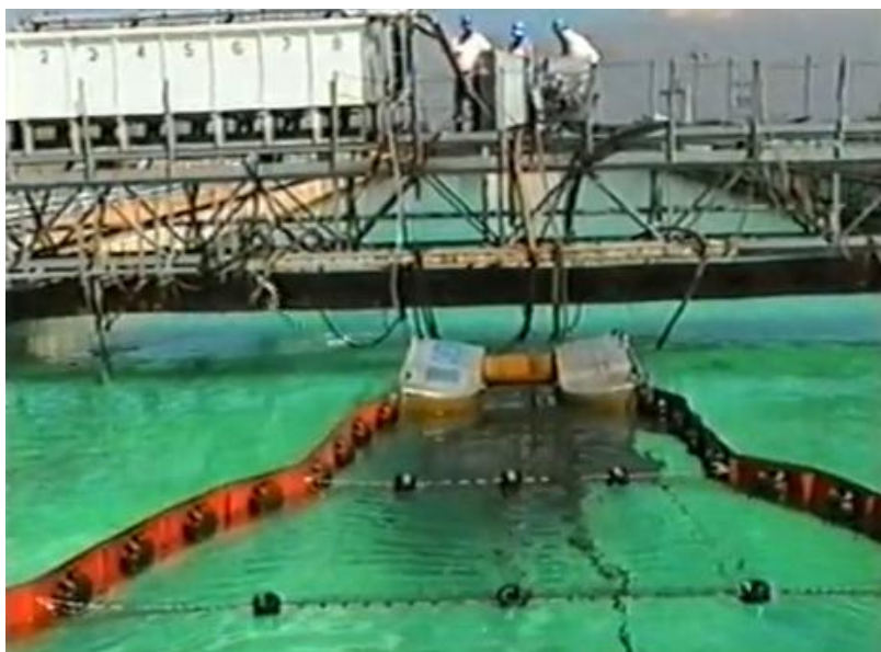
Figure 2-8. Pilot test of the “Big Crew” oil skimmer with floating boom (Omsett, 2010).
