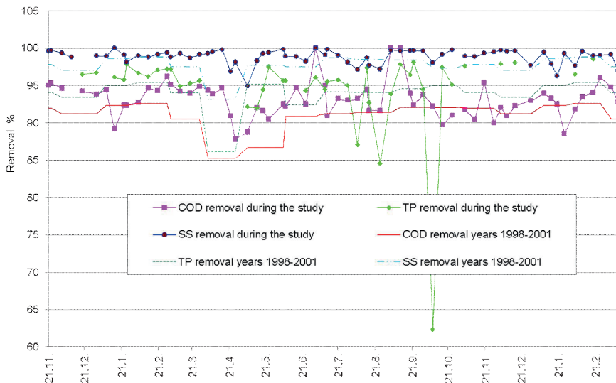
Figure 3.6 COD, SS and total phosphorus removal of the whole plant (including the tertiary filtration) during the study and on average during the three preceding years.
