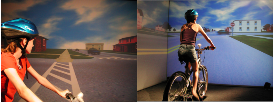
Figure 4.2: Photographs of the bicycling simulator. Note that the visual angles are correct from the viewpoint of the rider
