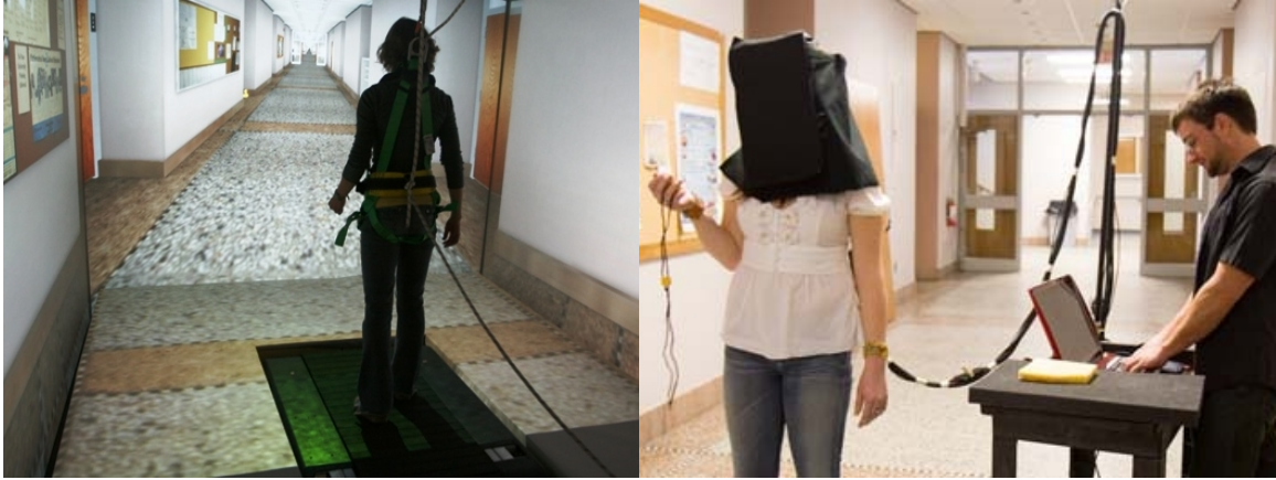
Figure 1.2: Virtual reality setups for behavioral studies with large projection screens (left) and HMD (right) used in Hank virtual reality laboratory.
