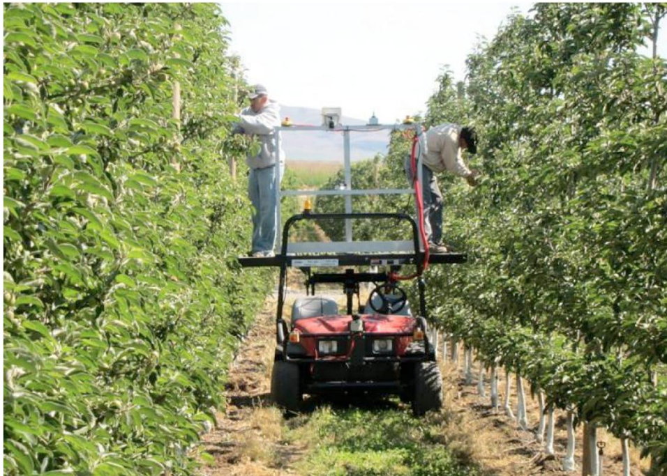
Figure 2.3 Farmers can perform thinning, pruning, or other operations on the platform of an autonomous vehicle developed by CASC project (Bergerman et al., 2012).
