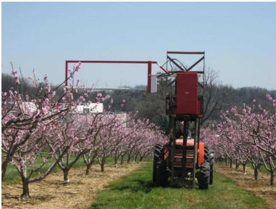
Figure 2.1 Darwin string thinner attached to a tractor during operation on vase-shape peach trees (Courtesy of Tara Baugher from PSU).
