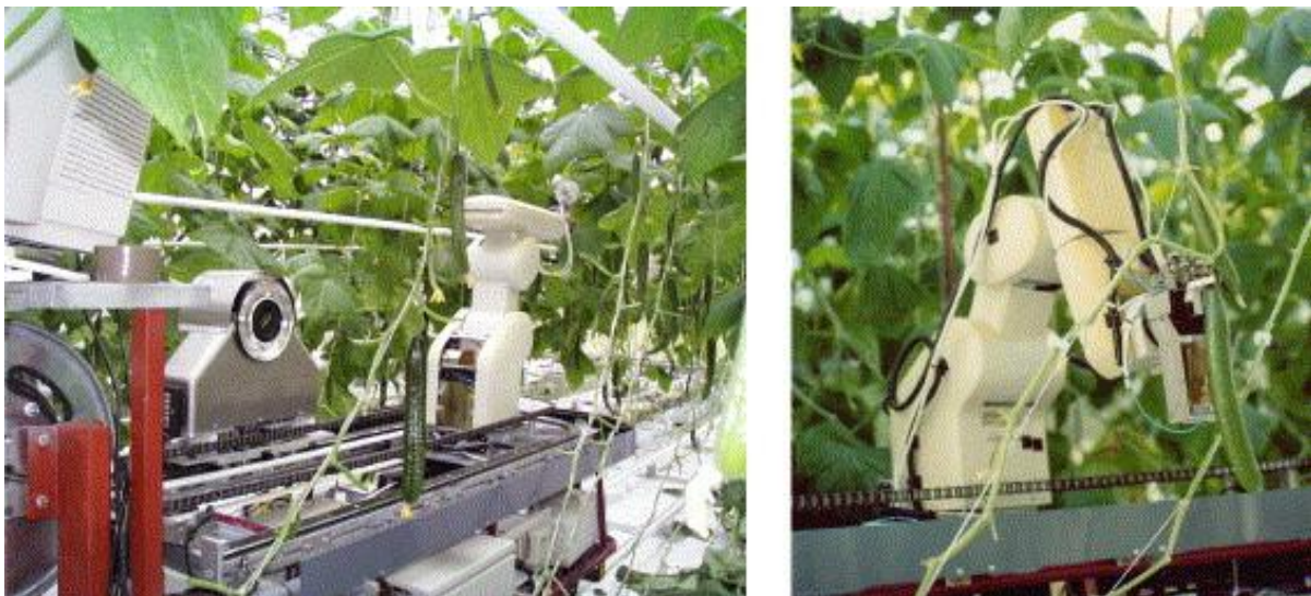
Figure 2.6 Field test of a cucumber harvesting robot (Van Henten et al., 2003b).
