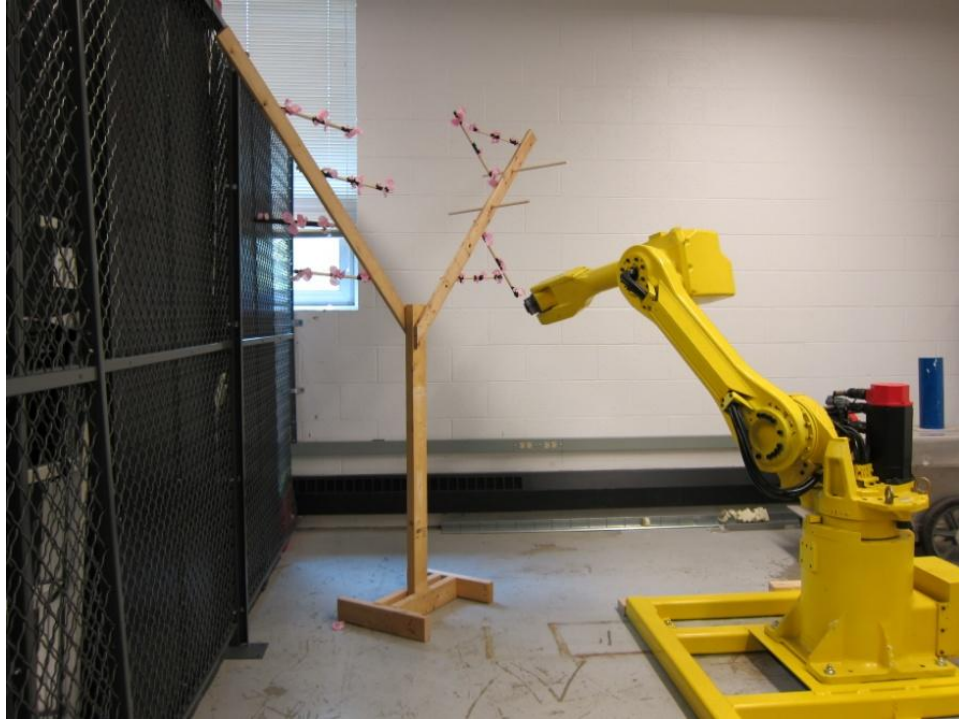
Figure 2.4 FANUC M-16iL industrial-grade manipulator with a model tree.
