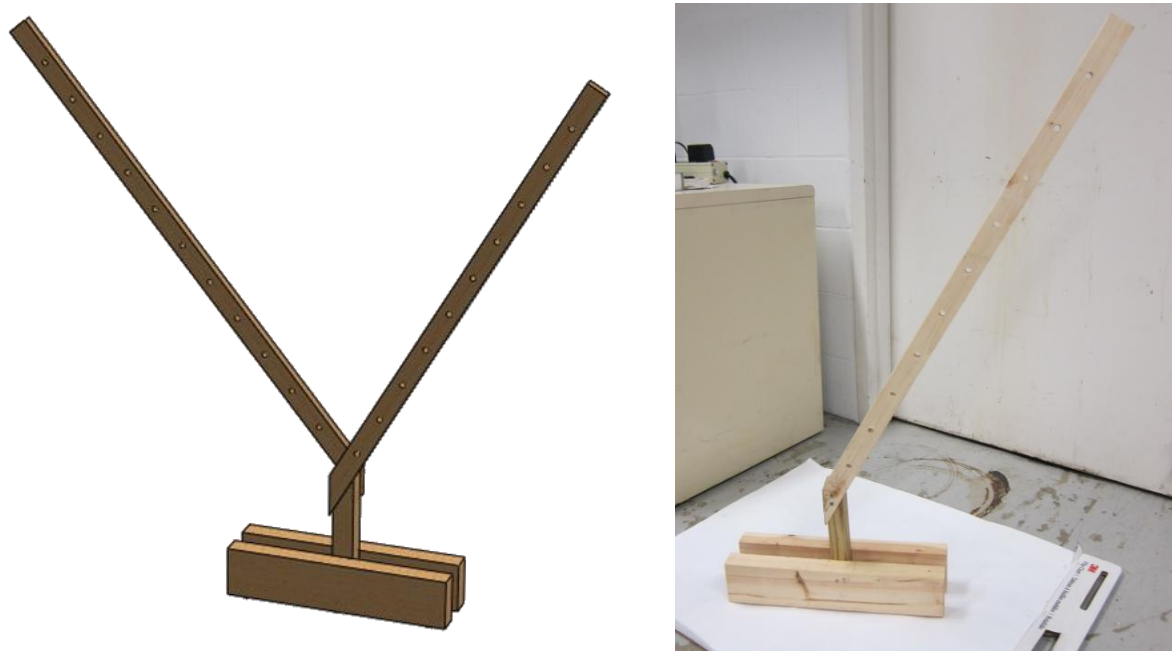
Figure 3.4 Left: model tree designed using CAD software SolidWorks ® . Right: prototype of the design.
