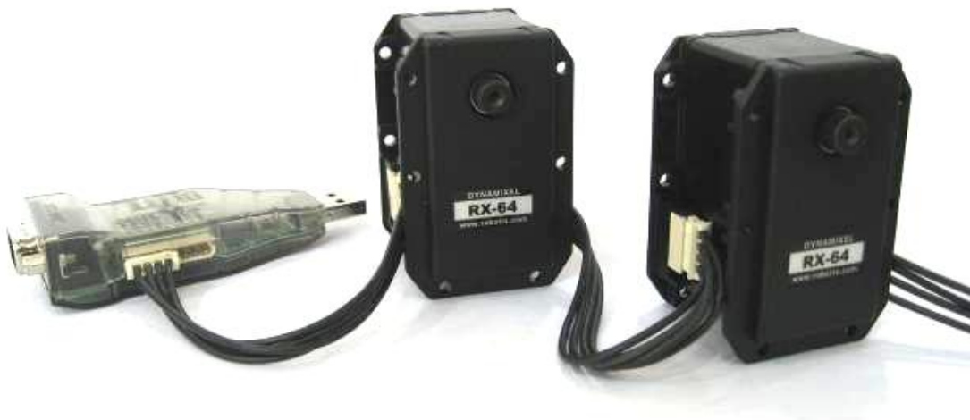
Figure 3.7 ROBOTIS ® motor controller USB2Dynamixel and two networked servomotors RX-64 (ROBOTIS, 2006).
