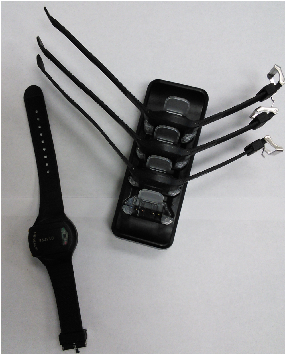
Figure 3.3: Geneactiv wristband system. Records 3D-accelerometer measurements at up to 100 Hz for up to one week. Does not have wireless capabilities.
