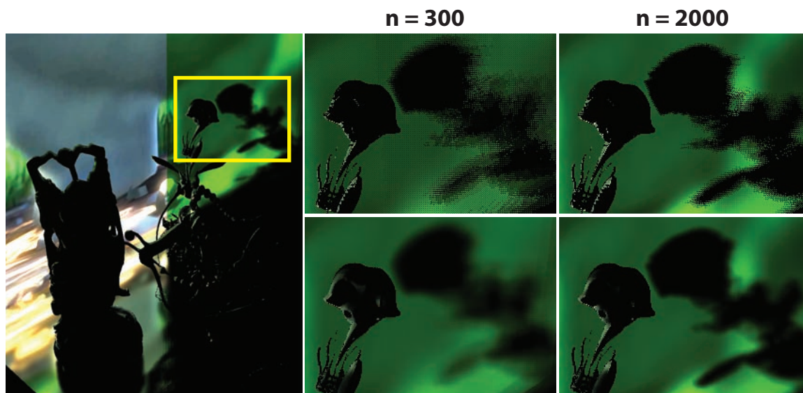
Figure 5.16: With sharp BRDFs, simple binary visibility queries may require many VPLs to produce artifact-free results. Here, the limited set of VPLs produces banding and interleaving artifacts with binary visibility queries (top). Querying using filtered variance values yields much better results (bottom).
