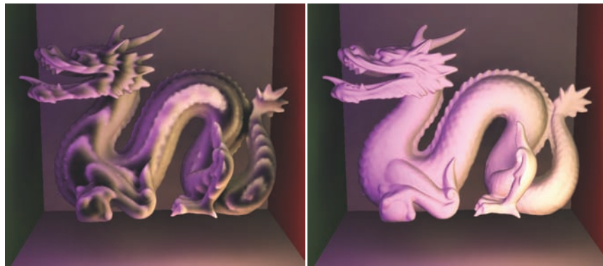
Figure 5.12: A dragon with self-occlusion artifacts due to limited voxel resolution. A bias helps alleviate the problem.
