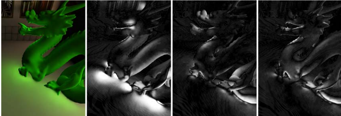
Figure 4.5: Temporal coherence between two successive animation frames. From left to right: the brightened indirect illumination, frame-to-frame difference using RSMs with 256 VPLs, difference using image-space radiosity, and difference using hierarchical image-space radiosity.
