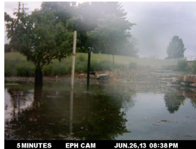
Figure A.9. Infiltration and rainfall continue on June 26, 2013: a) 175, b) 180, c) 185, and d) 190 minutes after start of rainfall. Plant Cam entered sleep, so not subsequent photos of this event were recorded.
