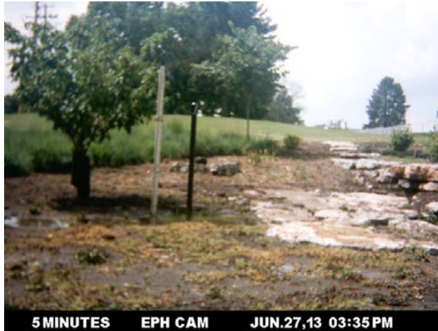
Figure A.15: The rain garden has gone from ponded water to no water ponded in about an hour. Also, the groundhog appears in the photo (d).
