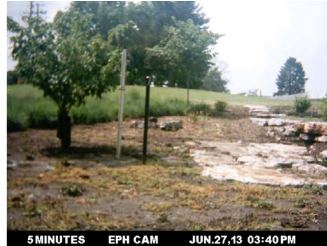
Figure A.15: The rain garden has gone from ponded water to no water ponded in about an hour. Also, the groundhog appears in the photo (d).
