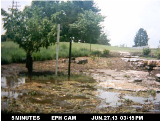
Figure A.14: Much of the surface showing and only micropools holding water. Photos are a) 30, b) 35, c) 40, and d) 45 minutes after the start of rainfall.
