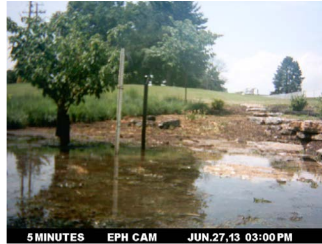
FigureA.13. Ponded water infiltrates after a rain event on June 27, 2013: a) 10, b) 15, c) 20, and d) 25 minutes after the start of rainfall.
