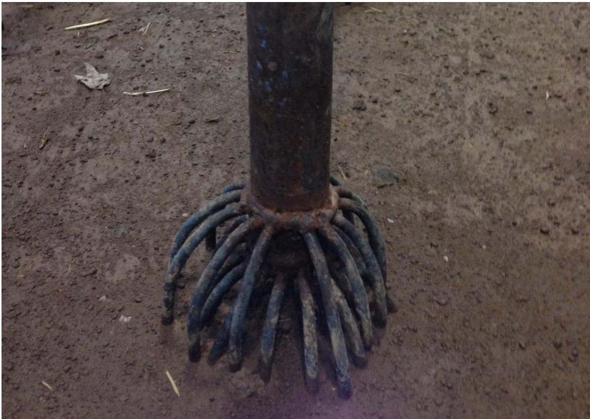
Figure 3-4 Simulated corn roots driven into soil prior to placement in rainfall simulator
