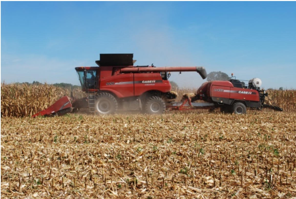
Figure 1-1 Single pass combine and large square baler system
