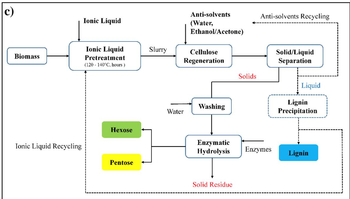
**Figure 7.** Pretreatment process flow chart illustrating paths of structural sugars and lignin
