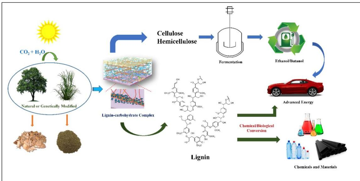
**Figure 1.** Schematic illustration of the production of fuels and chemicals from lignocellulosic biomass
