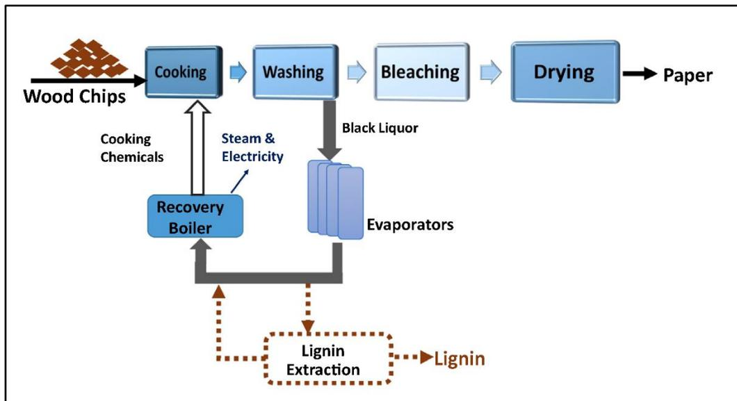
**Figure 6.** A typical Kraft pulping process (Haddad et al., 2017)
