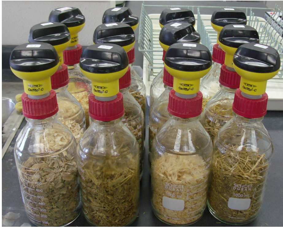
Figure 2. OxiTop® bottles used for lab-scale evaluation of swine tissue degradation and oxygen uptake.
