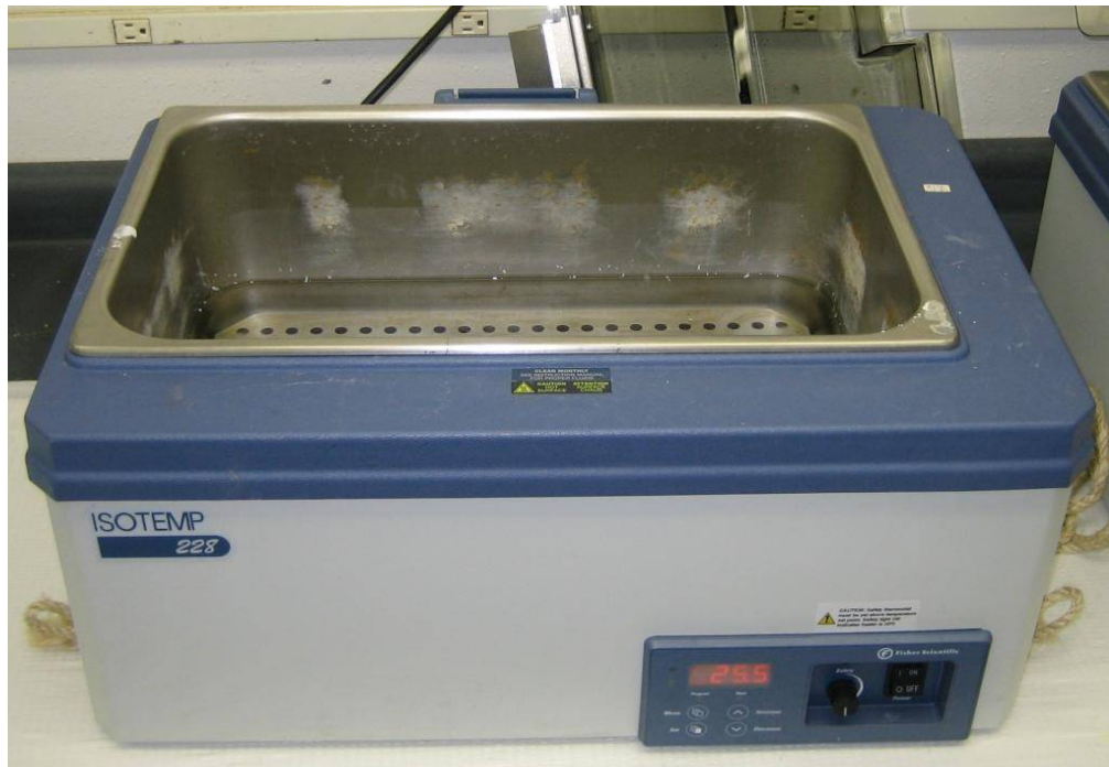
Figure 9. Fisher Scientific water bath used for OxiTop® bottle incubation.
