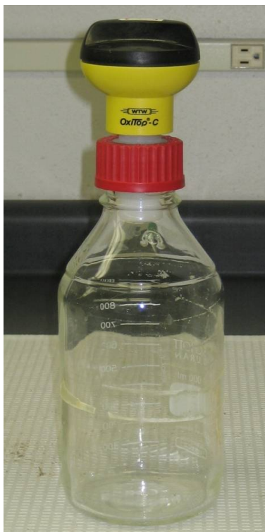
Figure 7. OxiTop® bottle with pressure sensor head used for respiration tests.
