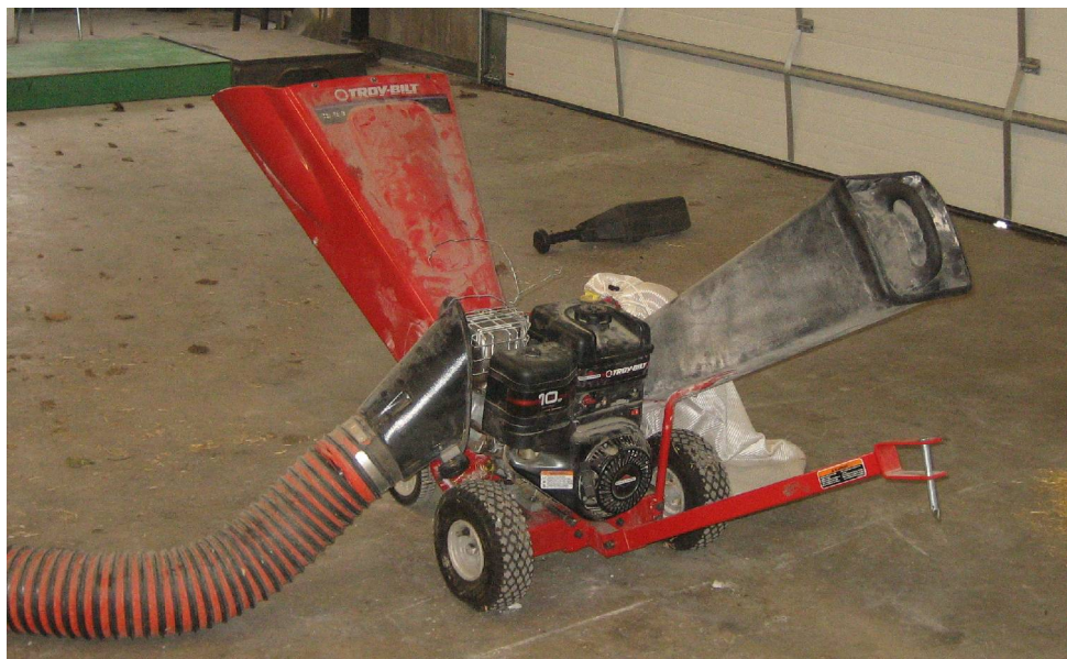
Figure 5. Troy-Bilt wood chipper used for envelope material particle size reduction.
