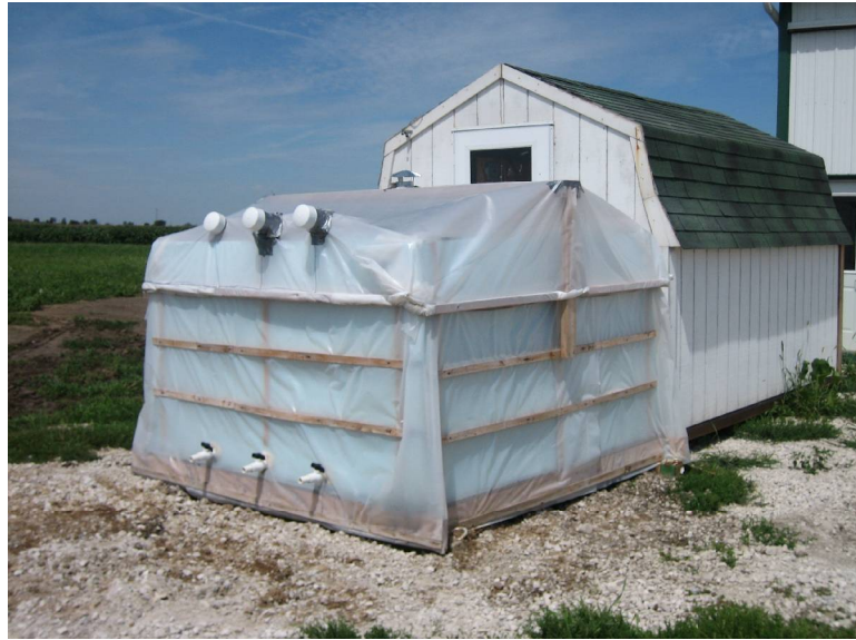
Figure 1. Field-scale biosecure mortality composting test unit with plastic biosecurity layer.
