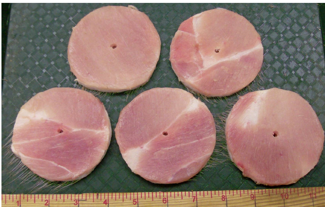
Figure 6. Swine tissue samples used during lab-scale experiment cut to uniform size using a hole saw.
