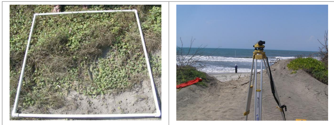
Figure 13. 1 m 2 quadrat to identify and quantify vegetation (left) and topographic profile along dunes, the latter using an AT G6 Topcon level (right).
