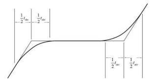
Figure 3.4: Acceleration-deceleration cycle for a single stop
