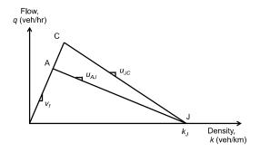
Figure 3.3: Fundamental diagram
