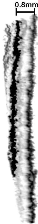
Figure 16: Stationary HRXT measurements showing the images after an angular displacement of the sample to compute the radius of curvature for the sample warpage.
