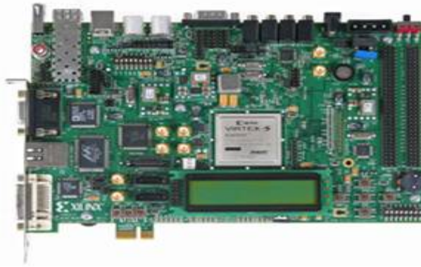
Figure 3.1: Virtex-5 FPGA Board; Device : XC5VFX70Tff1136
