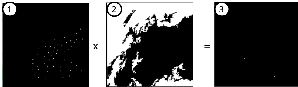
Figure 33: 1) GT skin image 2) Algorithm output non-skin image with non-skin in white; 3) Algorithm missed non-skin locations
