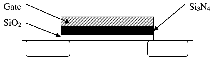
Figure 1.8 Charge Trapping Devices (MNOS device)
