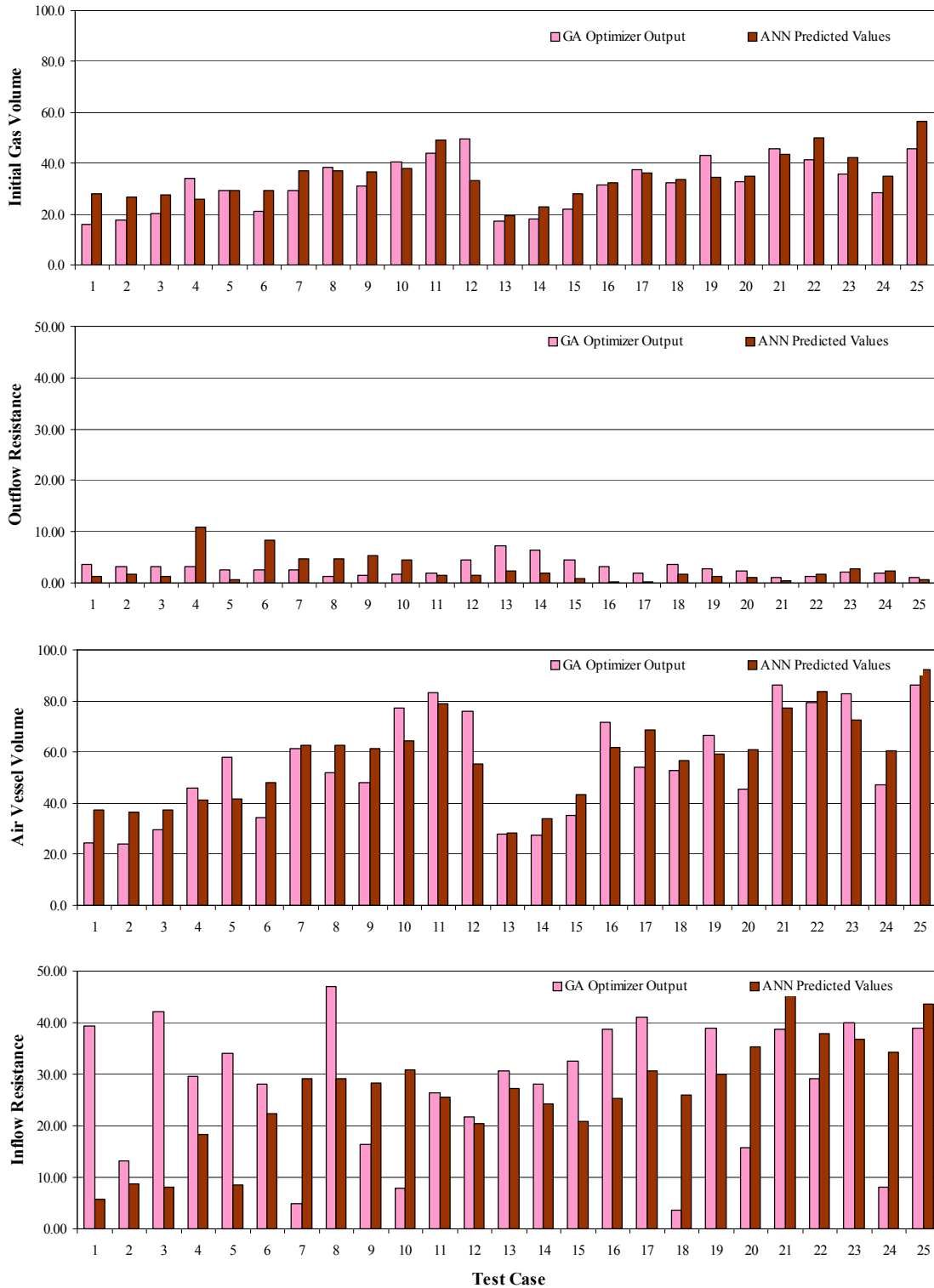
Figure 2.6 ANN predicted air vessel parameters vs. GA optimizer values
