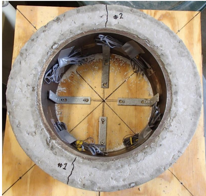
Figure 5-20: Shrinkage Cracking Occurring as Two Cracks in a Confined Shrinkage Ring
