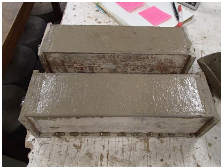
Figure 4-21: Mortar Cast into Molds to be used for ASR Testing
