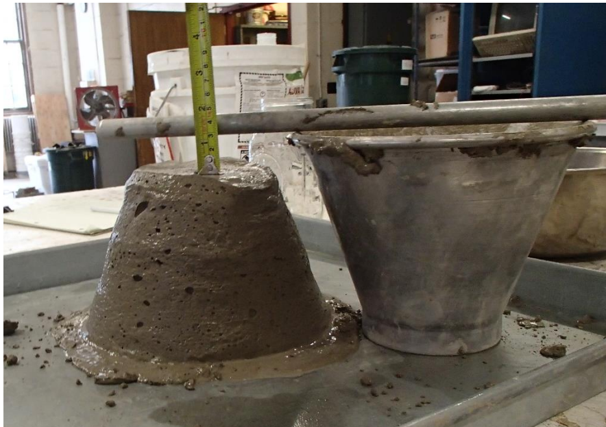
Figure 4-6: The “Slump” Measurement Being Taken on Concrete Containing a HRWR Dosage of 16 oz./cwt
