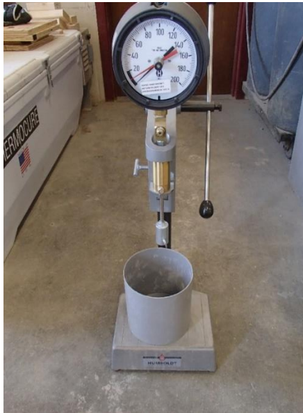
Figure 4-12: Acme Penetrometer Used to Measure Initial and Final Set Time of Concrete Mixtures & Various Penetrometer Needle Sizes
