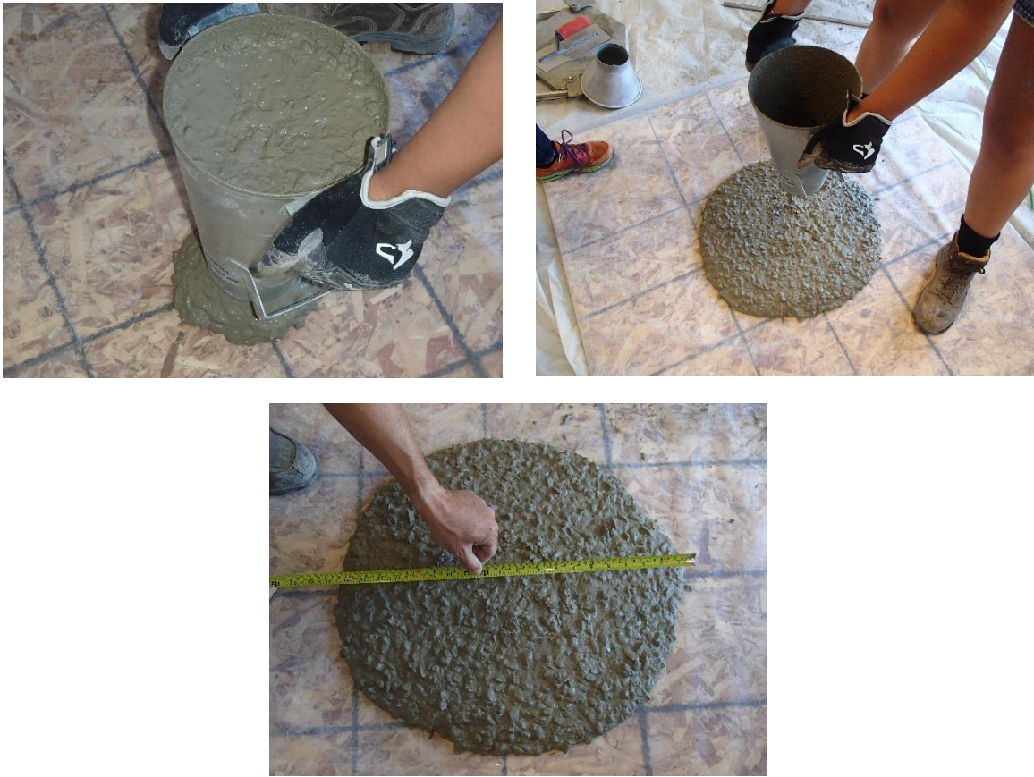
Figure 4-9: Lifting of Spread Test Mold and Measuring of the Resulting Circular Spread of Concrete
