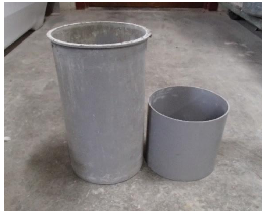
Figure 4-11: Plastic Cylindrical Mold Cut to be Used for Set Time Penetrometer Tests
