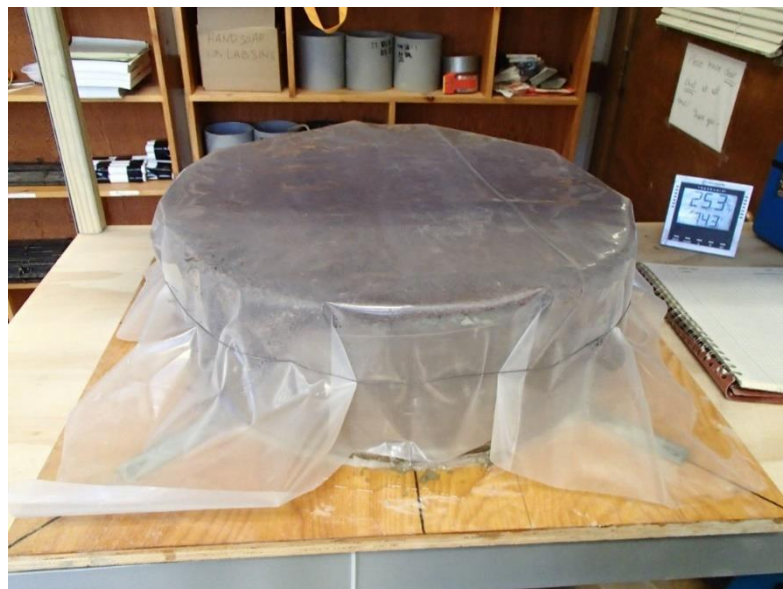
Figure 4-15: Wet Curing of the Top Surface of the Shrinkage Rings using Prewetted Burlap and Plastic Covering
