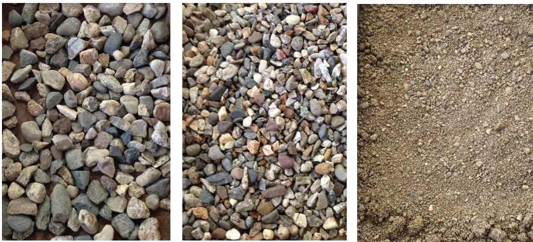
Figure 3-2: Depiction of Source 1 Aggregates. From Left to Right: 3/4” Coarse Aggregate, 1/2” Coarse Aggregate, Fine Aggregate
