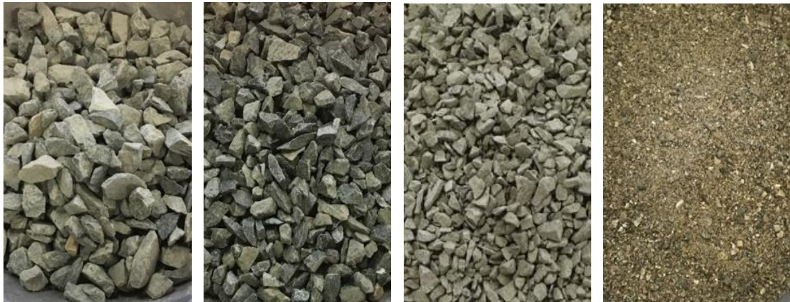
Figure 3-3: Depiction of Source 2 Aggregates. From Left to Right: 3/4" Coarse Aggregate, 1/2" Coarse Aggregate, 3/8" Coarse Aggregate, Fine Aggregate
