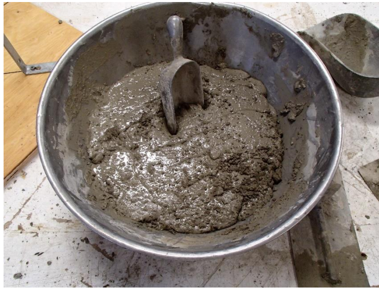
Figure 4-4: Concrete Hand-Mixed for HRWR Dosage Analysis Small-Scale Trial Batches
