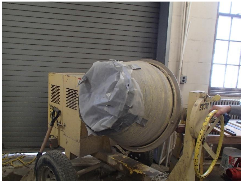
Figure 4-2: Concrete Batch in Machine Mixer During Rest Period with the Plastic Cover
