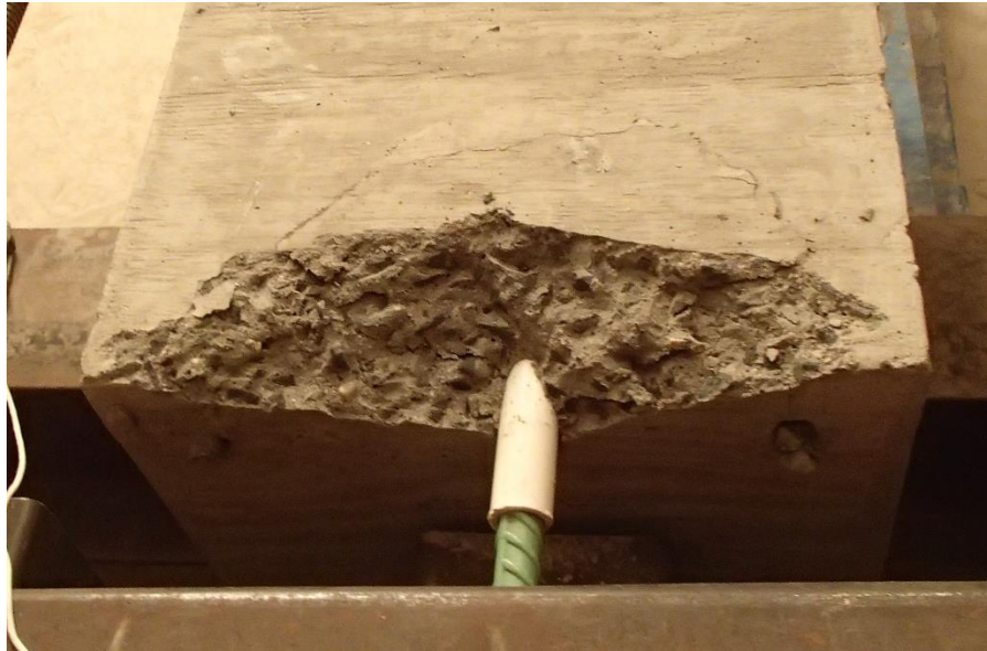
Figure 5-14: Concrete Cracking of Test Specimen 6-HD-6
