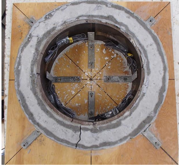
Figure 5-19: Shrinkage Cracking Occurring as One Crack in a Confined Shrinkage Ring
