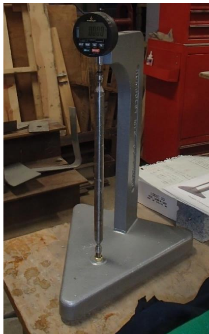
Figure 4-24: Length Comparator Shown Being Zeroed on Left and Taking a Reading of an ASR Specimen on Right
