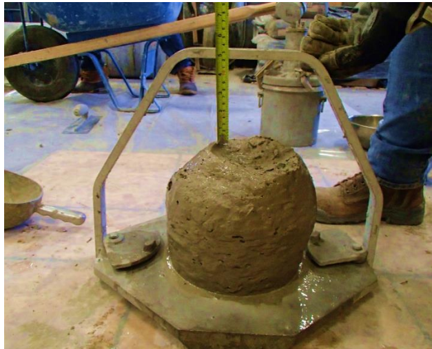
Figure 4-8: Measuring the Slump of a Concrete Mixture
