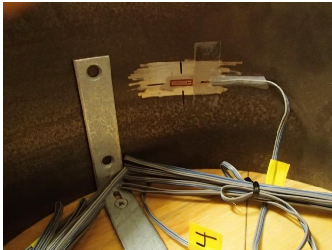
Figure 4-16: Bonded Strain Gauge to Steel Ring for Shrinkage Test
