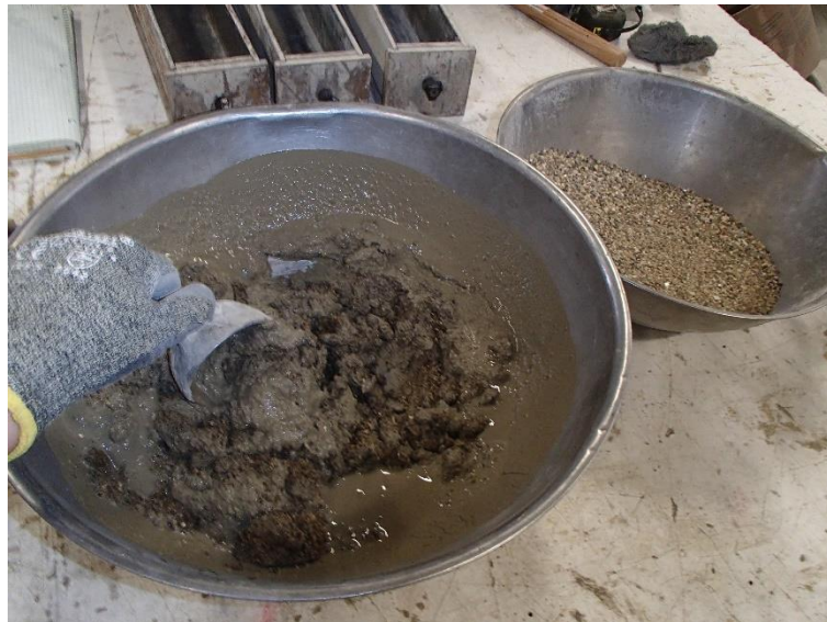
Figure 4-20: Hand Mixing the Mortar for ASR Testing
