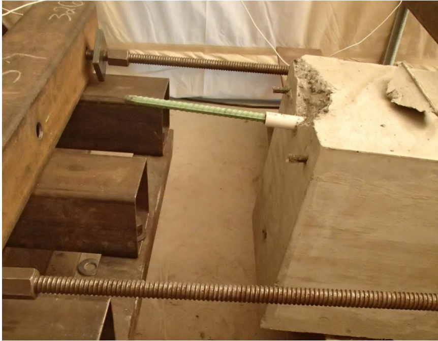
Figure5-11: Typical Failure of Bar Pullout Tests with No.4 Test Bar
