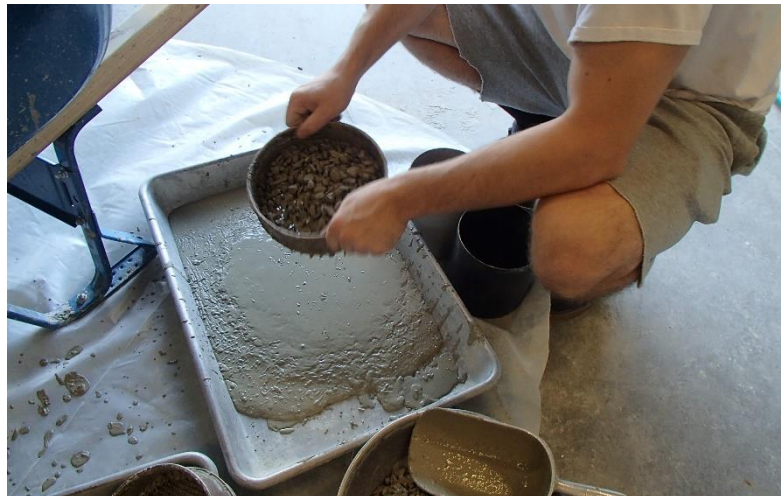
Figure 4-10: Sieving Coarse Aggregates out of Concrete to Form Mortar for Set Time Test
