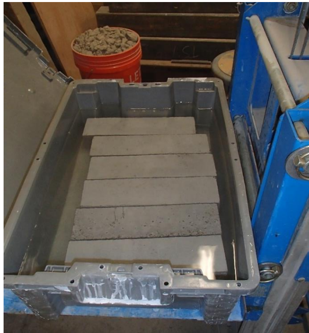
Figure 4-22: ASR Specimens Submerged in Sodium Hydroxide Solution
