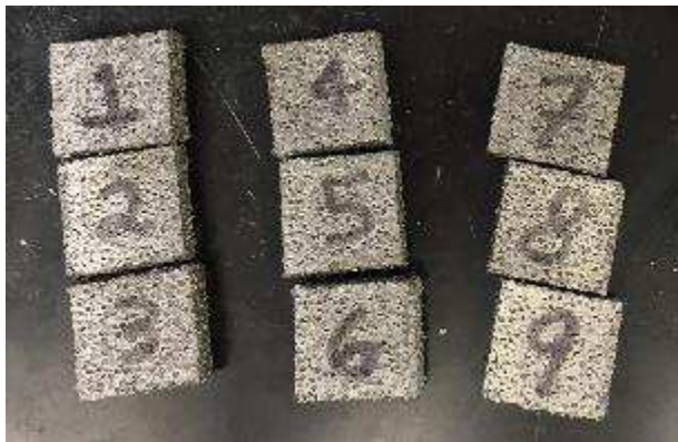
Figure 1.12: Samples of HS steel foam pre-impact testing
