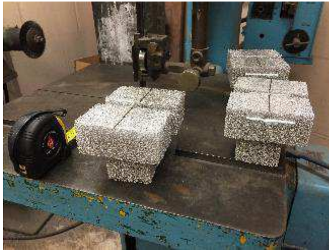
Figure 1.9: Pre-cut samples of aluminum foam
