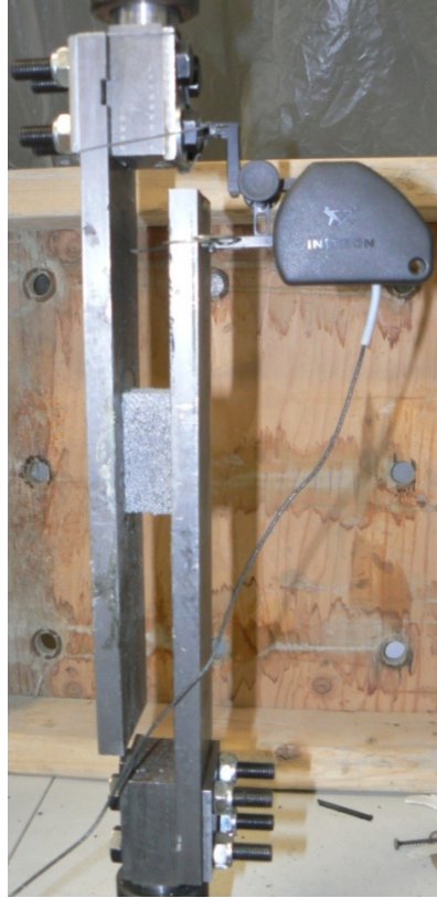
Figure 37: An image of the full shear test setup, ready to begin load application.
