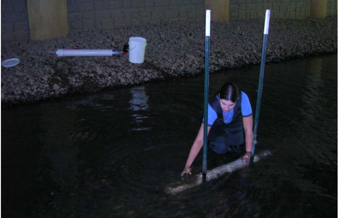
Figure 4-3) In-situ sediment trap implemented in the field
