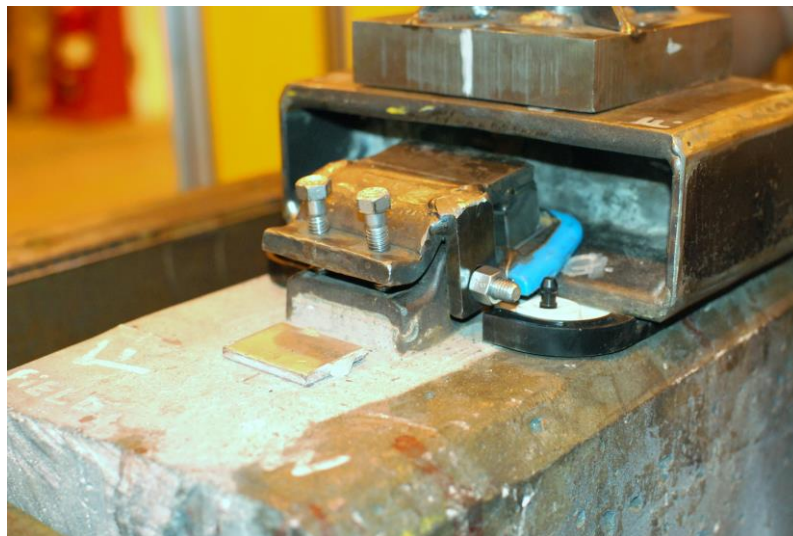
Figure 5.4 Fastening system used to connect the custom load fixture to the tie during ballast-box testing. Shown with the concrete tie section.
