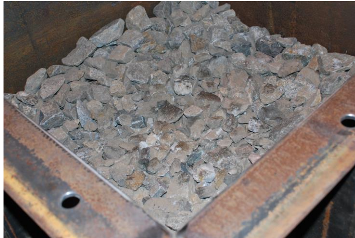
Figure 5.7 - Compacted bed of moderate ballast in a ballast box
