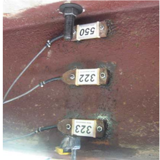
(b) Attached reusable strain gages
