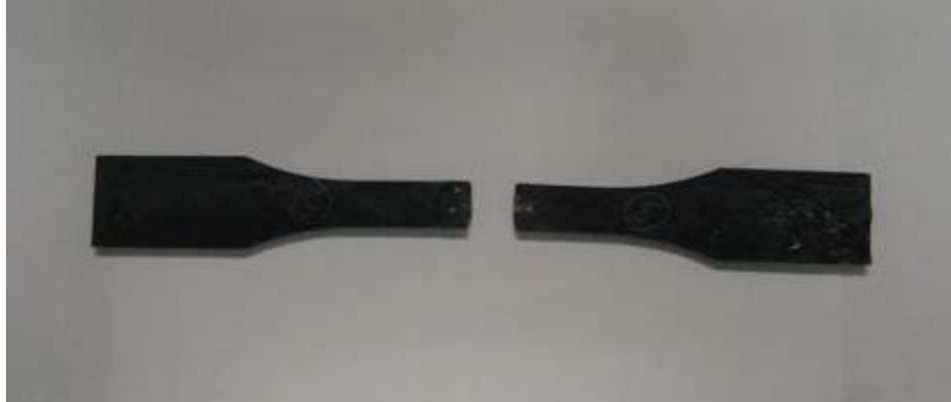
Fig. 2.7: Failure of Epoxy coupons
