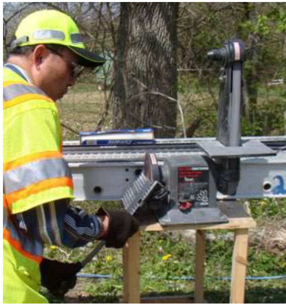
Fig. 5.16: Sanding laminate edges to obtain reverse taper
