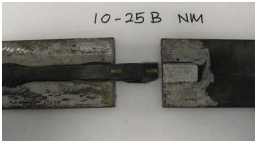
Fig. 2.10: Typical steel-epoxy interface debonding seen in normal modulus CFRP
