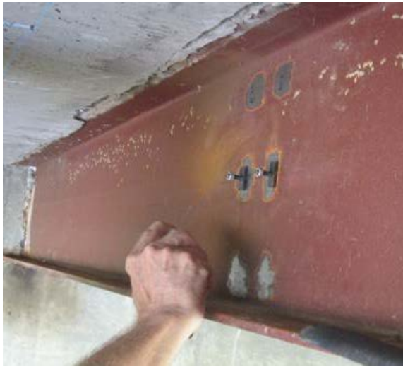
(a) Attaching tabs for gages
